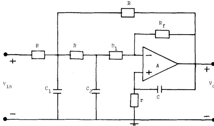
Figure 3. The improved Sallen-Key lowpass filter using the compensated inverting VCVS
