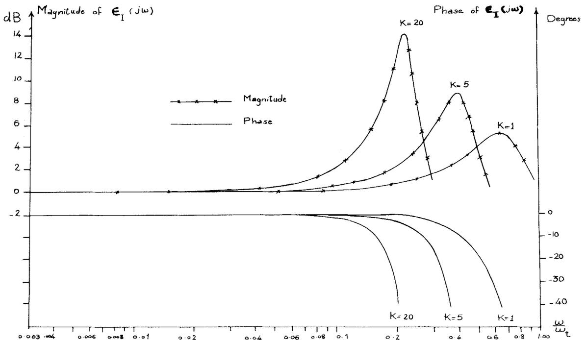
Figure 2. Magnitude and phase of  $\varepsilon_1(s)$  versus  $(\omega/\omega_t)$  with  $K$  taken as a parameter
