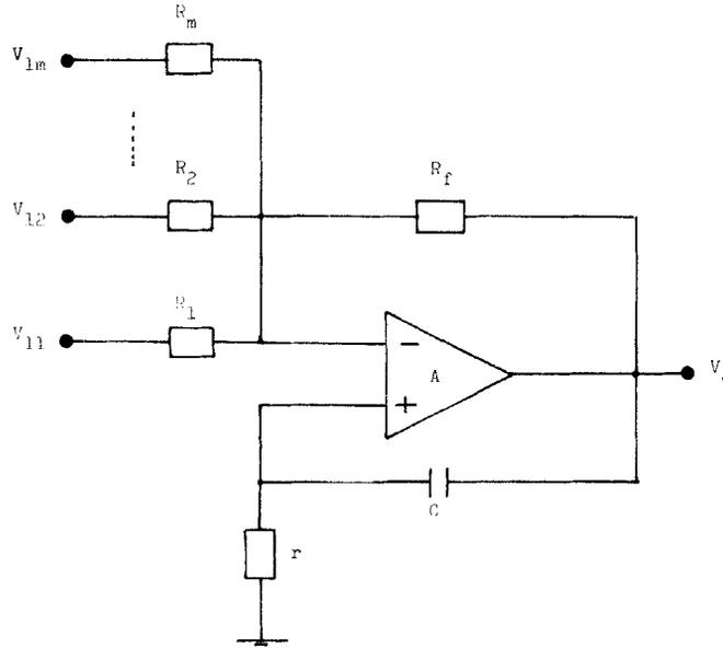
Figure 1. The proposed passive compensated inverting weighted summer
