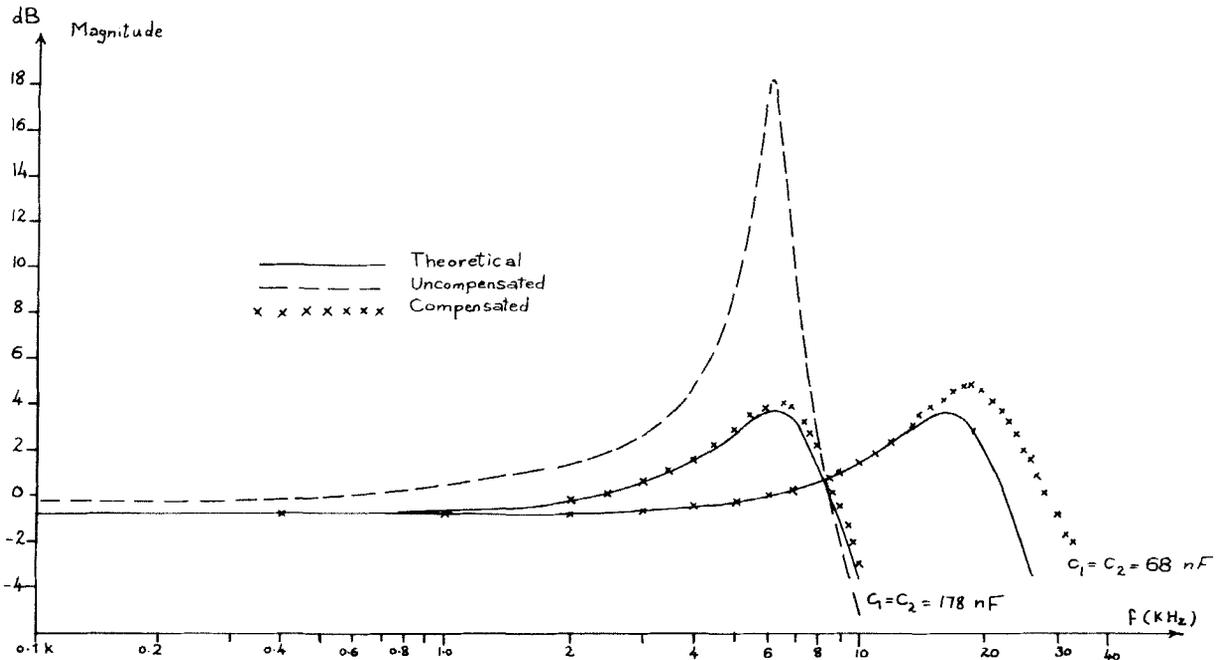
Figure 4. Magnitude vs. frequency response of the uncompensated and the compensated Sallen-Key lowpass filters
