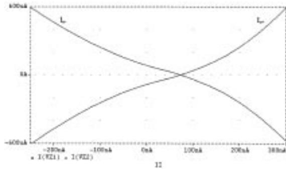
Fig. 6(a). The open loop DC transfer characteristics of the COA.
