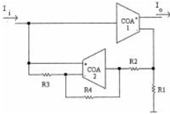
Fig. 11(b). The proposed COA-based active compensated amplifier.
