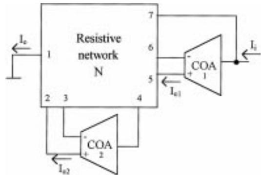
Fig. 10(b). The proposed generalized COA-based active compensated noninverting amplifier.
