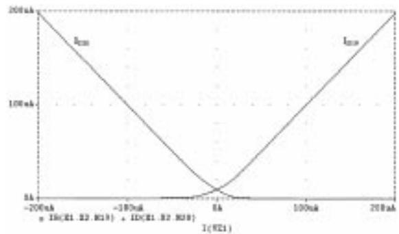
Fig. 6(e). The two current components forming  $I_{o-}$  and flowing through  $M_{19}$  and  $M_{20}$ .
