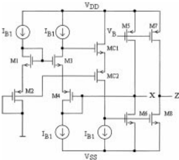
Fig. 7(a). Voltage offset compensated current follower.
