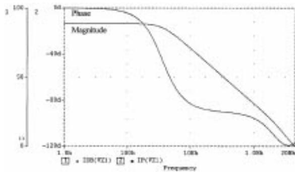
Fig. 8(b). The open loop gain of the modified COA.
