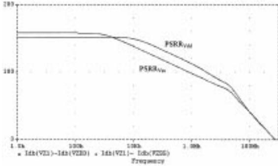
Fig. 6(g). The positive and the negative power supply rejection ratios of the COA.
