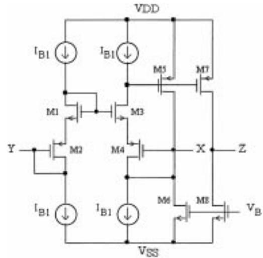
Fig. 3. Possible CMOS realizations of the CCII+ forming the input stage of the proposed COA.
