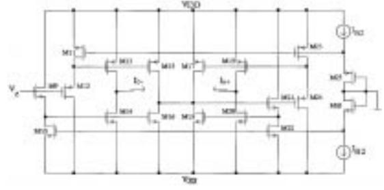
Fig. 4. The class AB floating transconductor used as the output stage of the proposed COA.
