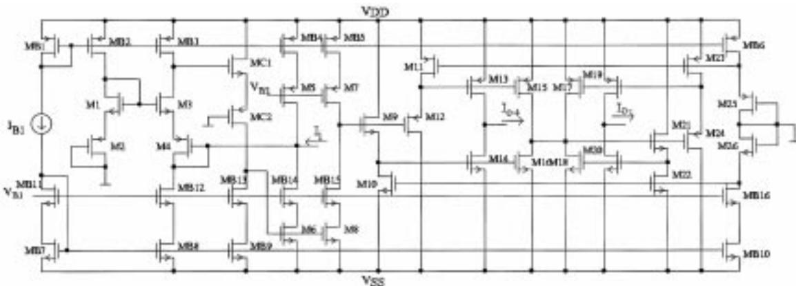
Fig. 7(b). The modified COA realization.
