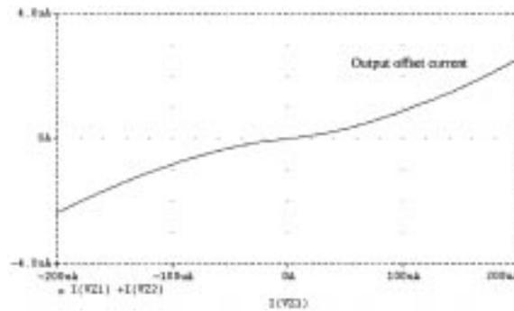
Fig. 6(b). The variation in the output current offset ( $I_{o+} + I_{o-}$ ) versus  $I_{o+}$ .
