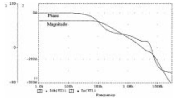
Fig. 6(f). The open loop AC transfer characteristics of the proposed COA.
