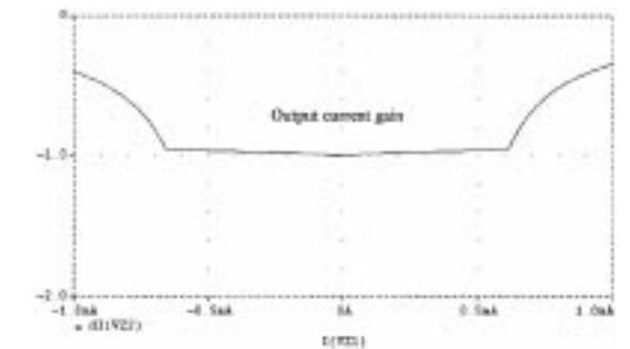
Fig. 6(c). The DC output current gain ( $I_{o-}/I_{o+}$ ) versus  $I_{o+}$ .
