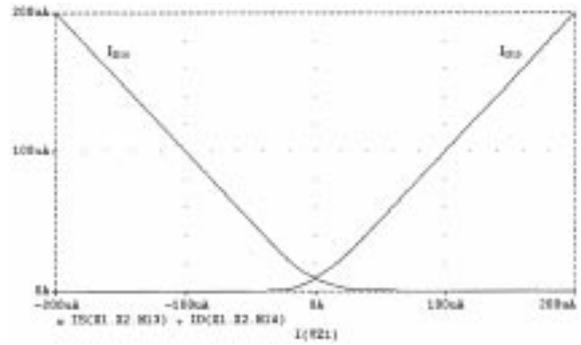
Fig. 6(d). The two current components forming  $I_{o+}$  and flowing through  $M_{13}$  and  $M_{14}$ .
