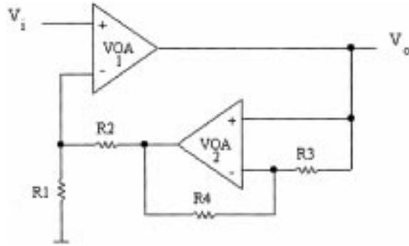
Fig. 11(a). The VOA-based active compensated noninverting amplifier given in [10].
