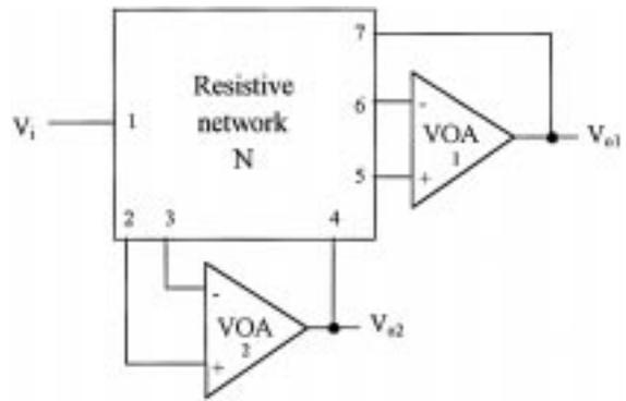
Fig. 10(a). The generalized VOA-based active compensated noninverting amplifier given in [9].
