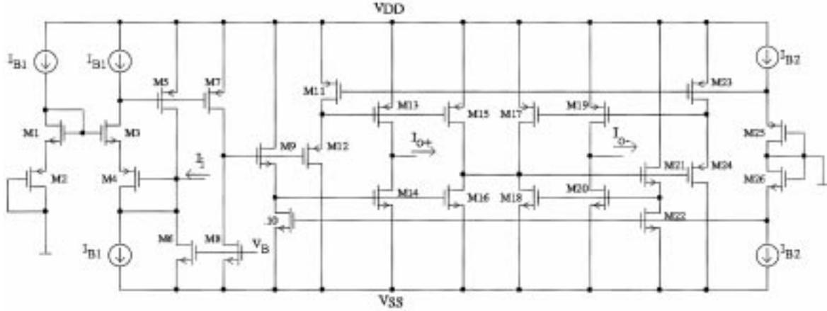
Fig. 5. The complete CMOS realization of the proposed COA.
