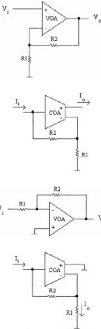
Fig. 9. The VOA-based amplifiers and their adjoint current mode amplifiers implemented using the COA.
