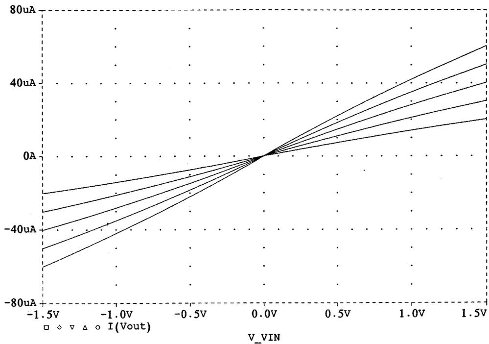
Fig. 8. Output current  $I_O$  against  $V_I$  with different values of  $I_B$ .
