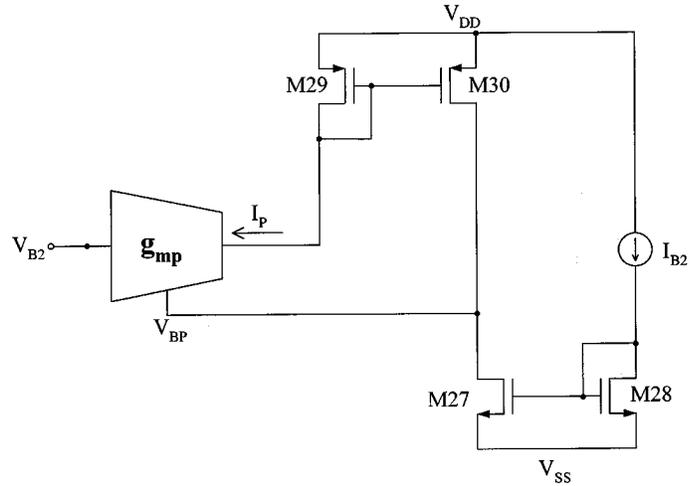
Fig. 5. The biasing circuit of the  $P$  part.
