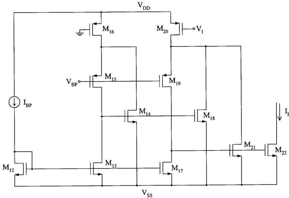
Fig. 3. The  $P$  part of the proposed transconductor.
