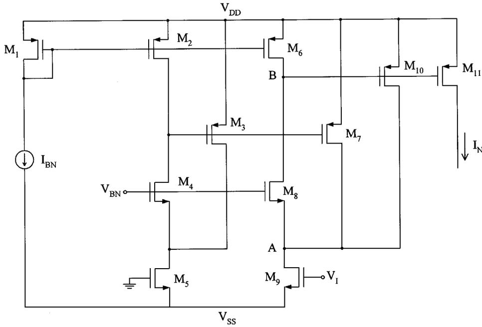
Fig. 2. The  $N$  part of the proposed transconductor.
