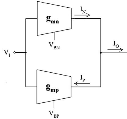
Fig. 1. The block diagram of the proposed transconductor circuit.
