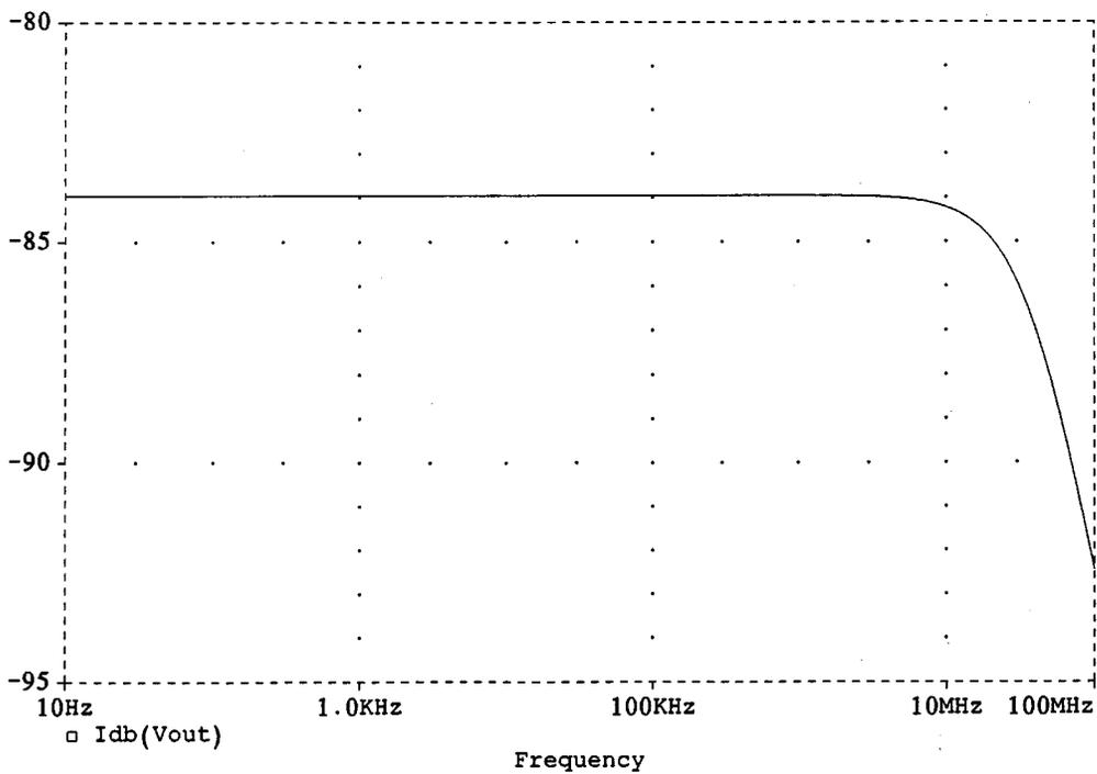
Fig. 9. Short-circuit frequency response at the output terminal when  $V_I = 1 V$ ,  $I_B = 50 \mu A$ .
