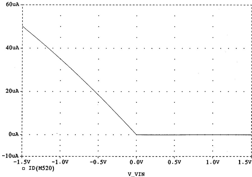
Fig. 7. The currents  $I_P$  against  $V_I$  when  $I_B = 50 \mu\text{A}$ .
