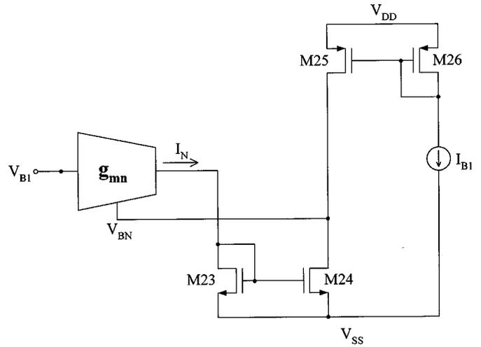
Fig. 4. The biasing circuit of the  $N$  part.
