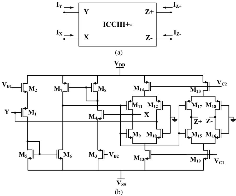
**Fig. 1** (a) Block diagram of ICCIII+- . (b) The proposed ICCIII+- CMOS realization
