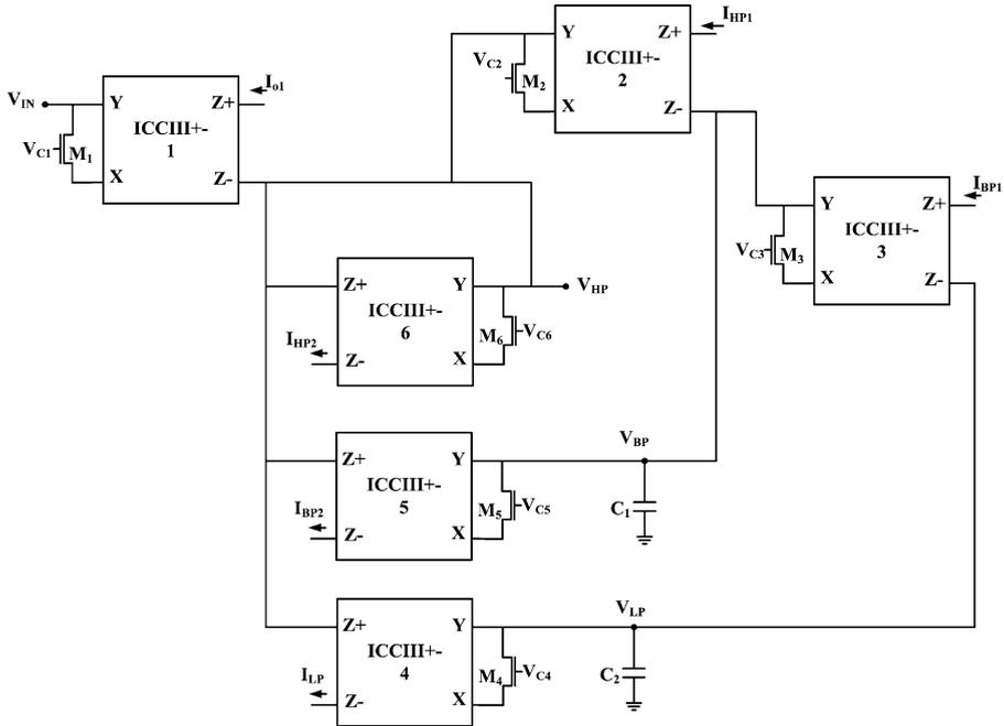
Fig. 7 The KHN MOS-C ICCIII+- filter circuit
