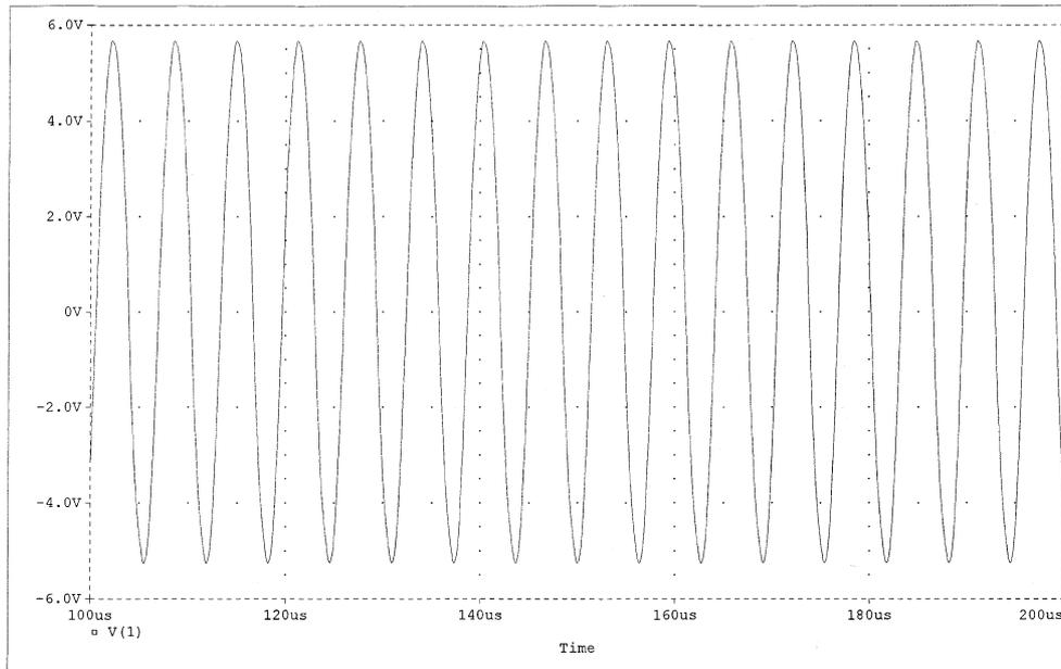
*Fig. 11.* The voltage waveform of the oscillator of Fig. 8(a) using MOS grounded resistors.
