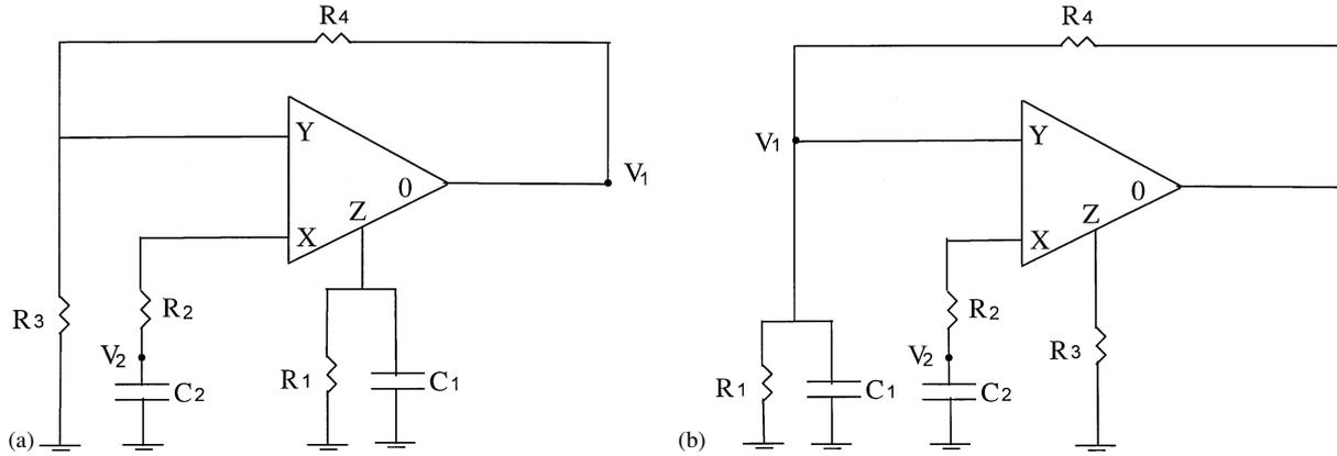
Fig. 3. Two modified grounded  $C$  oscillators using a single CFOA.
