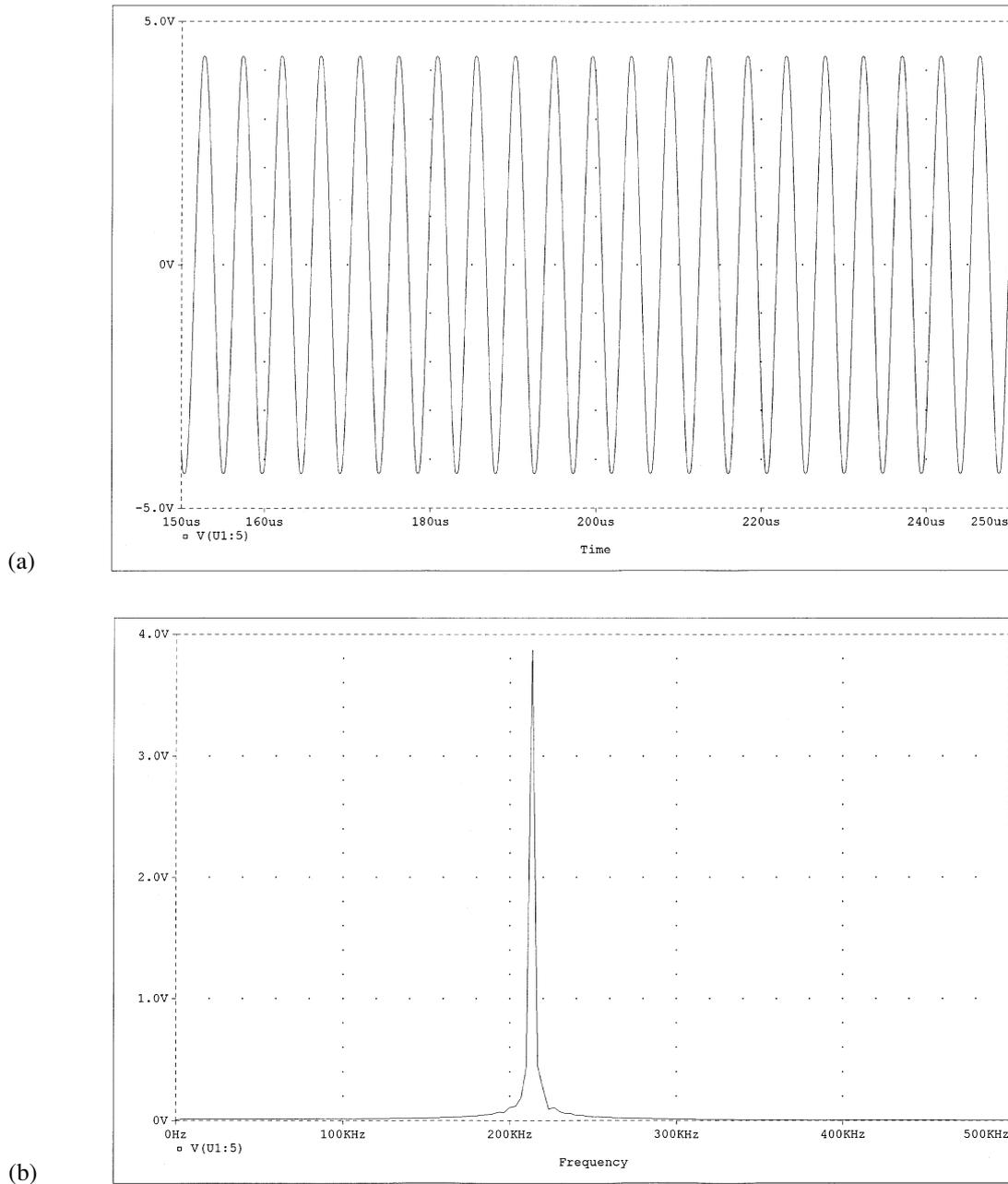
Fig. 4. (a) The output voltage waveform of the oscillator of Fig. 3(b). (b) The frequency spectrum of the oscillator of Fig. 3(b).
