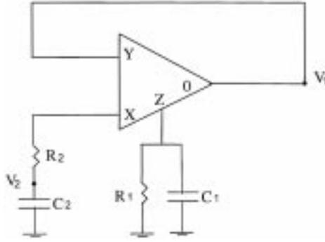
Fig. 1. The minimum passive component grounded  $C$  (or grounded  $R$ ) oscillator using a single CFOA.
