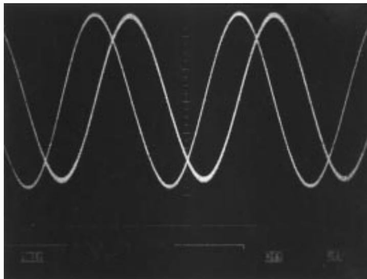
*Fig. 12.* Oscilloscope photograph of the  $V_1$  and  $V_2$  of the oscillator of Fig. 6(a). Vertical 1 V/div; horizontal 20  $\mu$ s/div.
