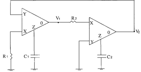
Fig. 2. The minimum passive component grounded  $C$  oscillator using two CFOAs.
