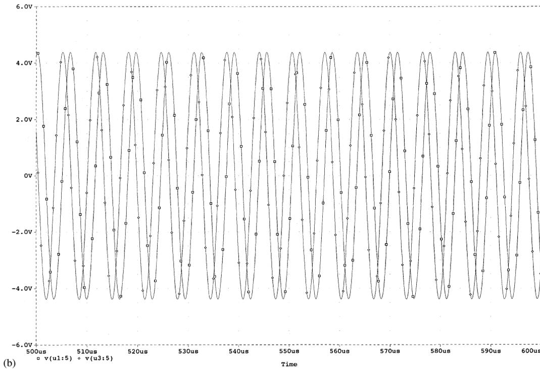
Fig. 9. (a) An alternative grounded  $C$ , grounded  $R$  oscillator using three CFOAs. (b) The  $V_1$  and  $V_2$  waveforms of the oscillator of Fig. 9(a).
