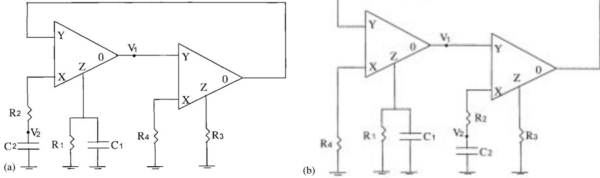
Fig. 5 Two new grounded  $C$  (or grounded  $R$ ) oscillators using two CFOAs.
