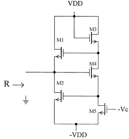
Fig. 10. The MOS grounded resistor [12].
