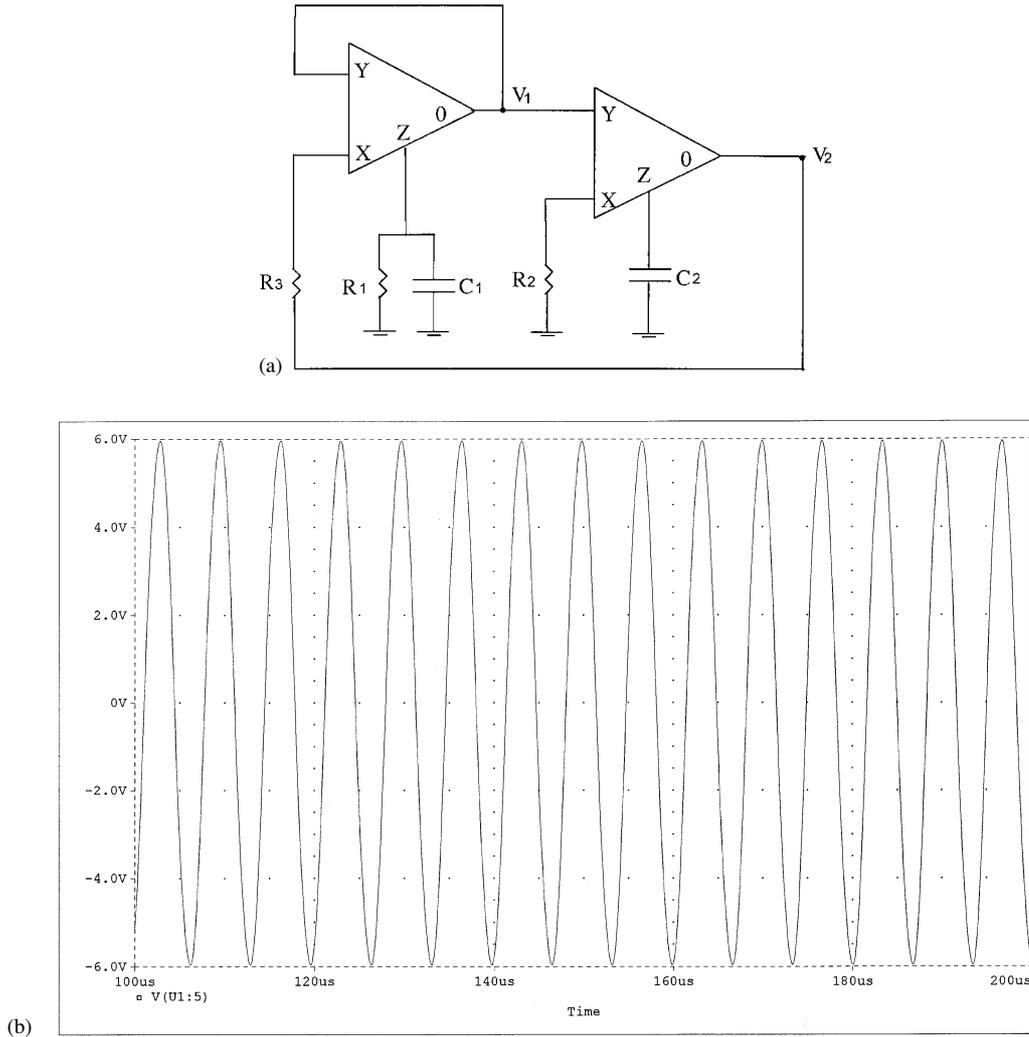
Fig. 6. (a) A new grounded  $C$  oscillator using two CFOAs. (b) The voltage  $V_1$  waveform of the oscillator of Fig. 6(a).
