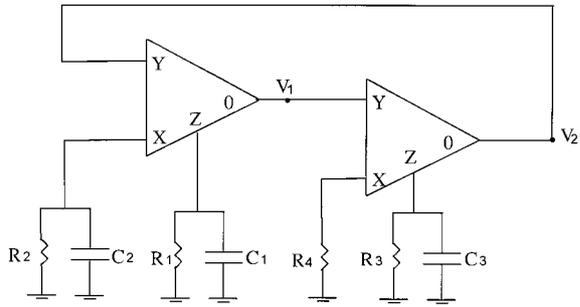
Fig. 7. A new grounded C, grounded R oscillator using two CFOA.
