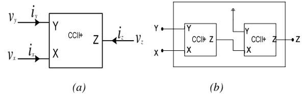
Figure 1. Symbol diagram (a) CCII+, (b) CCII-
