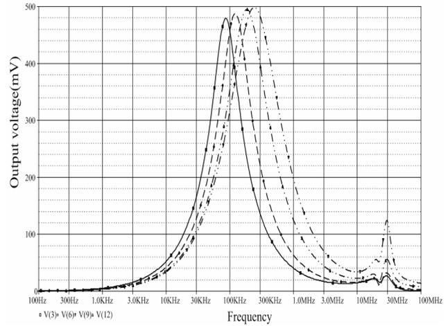
Figure 8. Frequency response of output voltage for different center frequency of the resonator circuit 87, 123, 188 and 243 KHz.
