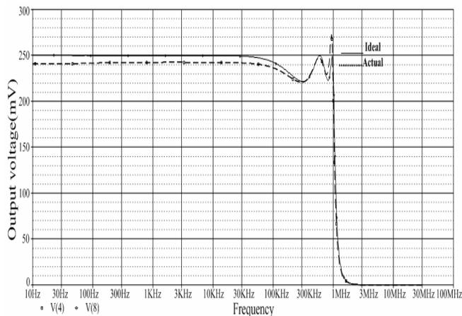
Figure 10. Ideal and actual frequency response of output voltage for the filter circuit.
