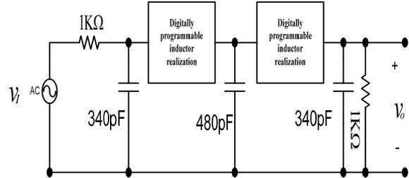
Figure 9. Fifth order Chebyshev low pass Ladder filter [11].
