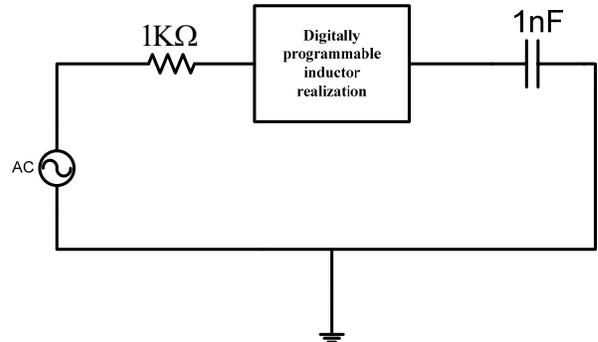
Figure 6. Passive circuit for a resonator.
