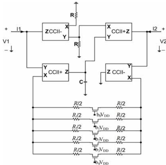
Figure 4. Digitally programmable Inductor realization
