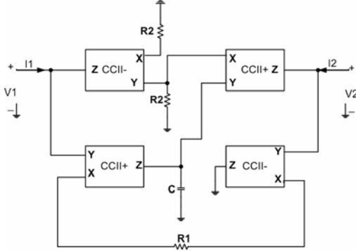
Figure 3. Floating inductor realization [9].
