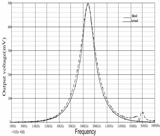
Figure 7. Ideal and actual frequency response of output voltage for the resonator circuit.
