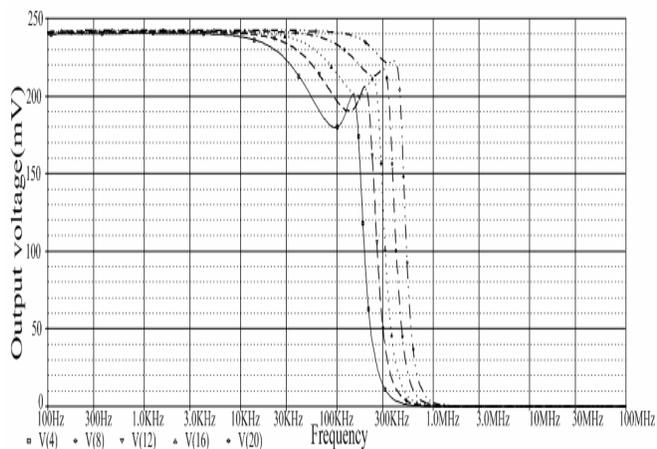
Figure 11. Frequency response of output voltage for different cut off frequency of the filter circuit 150, 196, 240, 300, 397 KHz.
