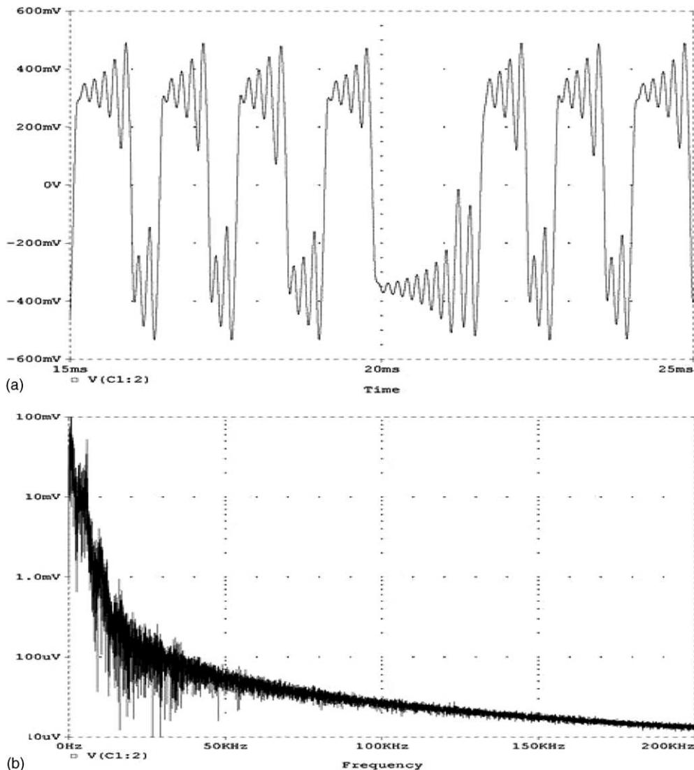
Fig. 11. (a)  $V_{C1}$  time waveform of Chua's circuit (double-scroll type) and (b) the frequency response of  $V_{C1}$  (double-scroll type).
