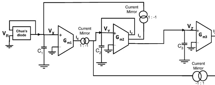
Fig. 6. The proposed block diagram of Chua's circuit.
