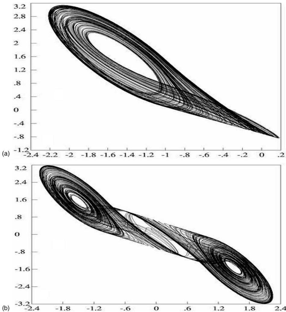
Fig. 9. (a)  $X$ - $Z$  numerical projection of Rossler attractor and (b)  $X$ - $Z$  numerical projection of the double scroll attractor.
