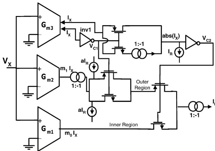
Fig. 3. The general block diagram of the controllable Chua’s diode.
