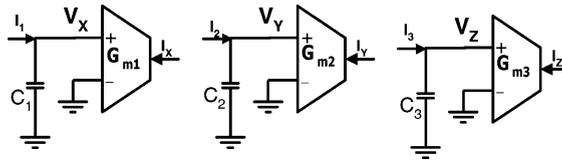
Fig. 2. Three simple current integrators.
