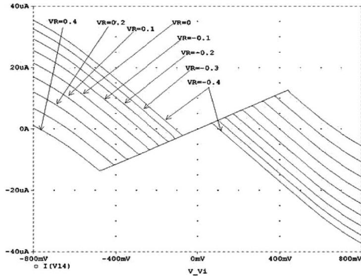
Fig. 5.  $I_0$ - $V_x$  projection of Chua's diode with different values of  $V_R$ .
