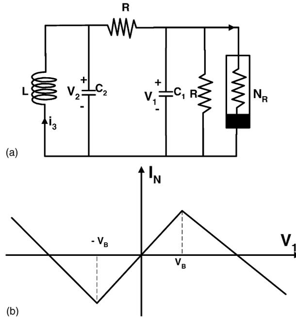
Fig. 1. (a) Chua's circuit and (b)  $I_N$ - $V_1$  characteristic of Chua's diode.
