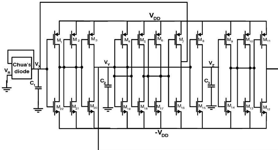
Fig. 7. The complete MOS circuit realization of Chua's circuit.
