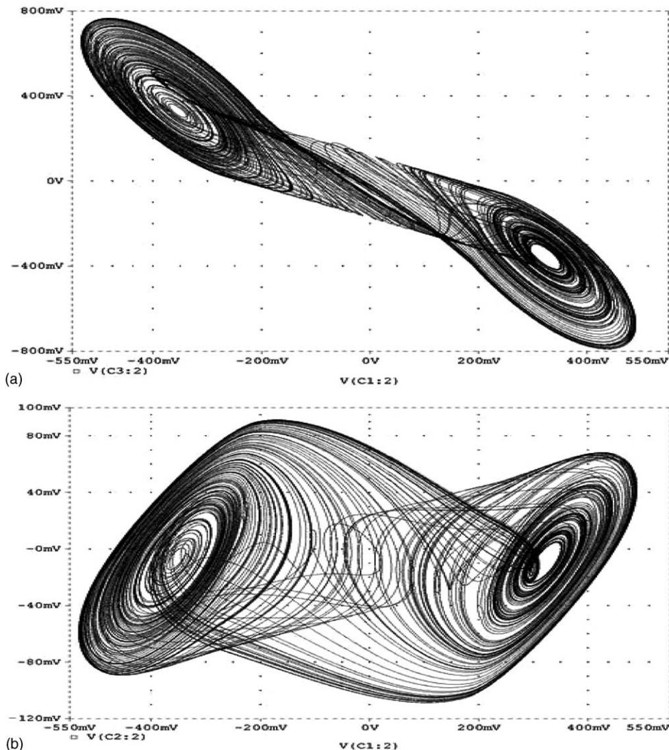
Fig. 10. (a)  $V_{C1}-V_{C3}$  projection of Chua's circuit (double-scroll type) and (b)  $V_{C1}-V_{C2}$  projection of Chua's circuit (double-scroll type).
