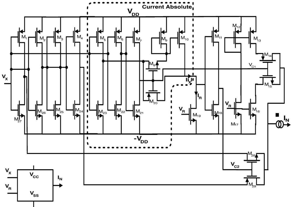
Fig. 4. The MOS circuit realization of proposed Chua's diode.
