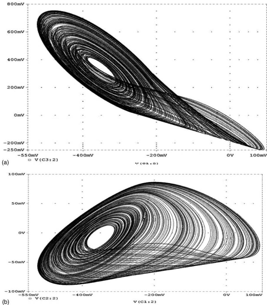
Fig. 8. (a)  $V_{C1}-V_{C3}$  projection of Chua's circuit (Rossler type) and (b)  $V_{C1}-V_{C2}$  projection of Chua's circuit (Rossler type).
