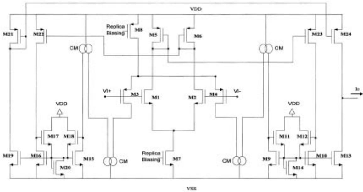
Fig. 7. Complete circuit diagram of the proposed TA.
