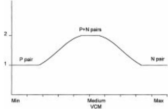
Fig. 3. Transconductance versus CM voltage of a rail-to-rail complementary CMOS stage.
