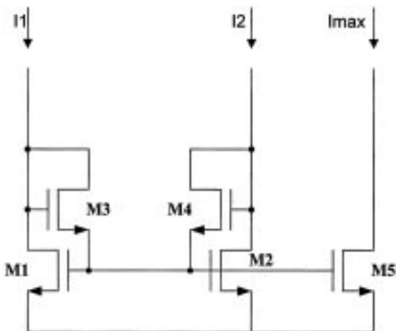
Fig. 4. Maximum selection circuit.
