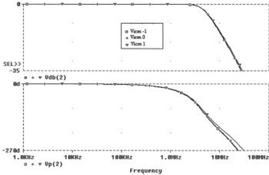
Fig. 13. Frequency response of the 2nd order filter for different values of the CM voltage.
