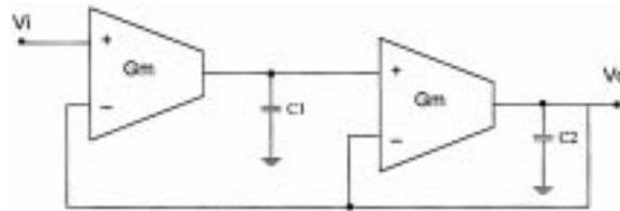
Fig. 12. Second order filter circuit diagram.
