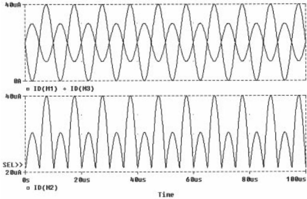
Fig. 6. Transient simulation of the maximum selection circuit.
