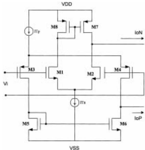
Fig. 2. Complementary CMOS rail-to-rail transconductance.
