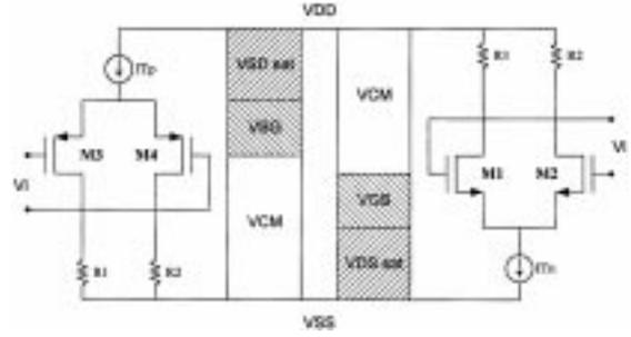
Fig. 1. CM range of P and N type CMOS differential stages.
