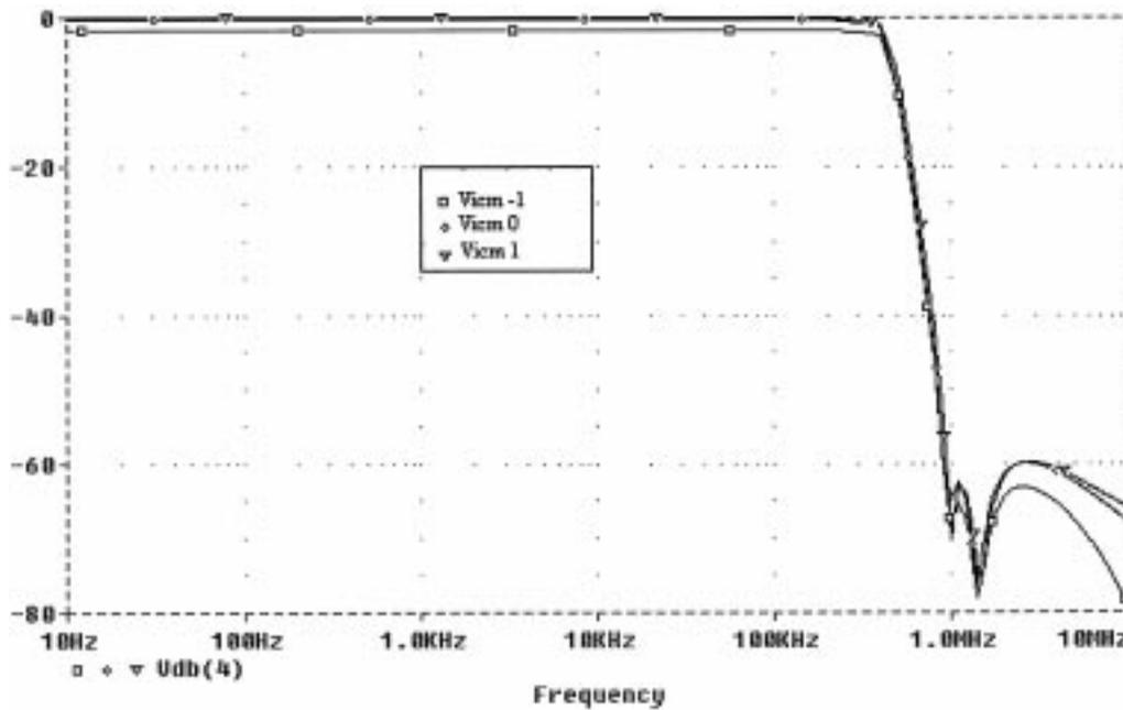
Fig. 15. Frequency response of the 5th order filter for different values of the CM voltage.
