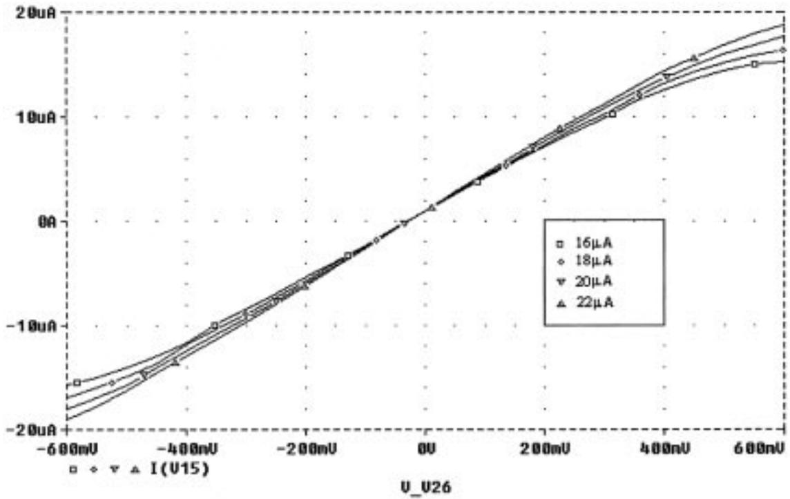
Fig. 9. Output current vs. step sweep of control current.
