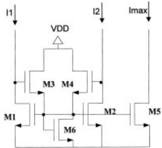
Fig. 5. Modified maximum selection circuit.
