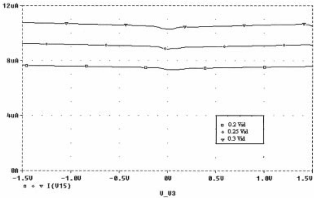
Fig. 10. Output current vs. a rail-to-rail sweep of the CM voltage at fixed differential input.
