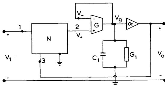
Fig. 1 General filter configuration
