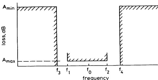
Fig. 1 Representation of geometrically symmetrical bandpass filters
