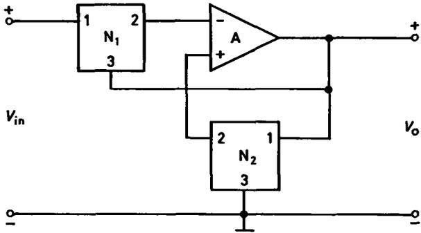
Fig. 1: The passive compensated noncanonic bandpass filter [5]
