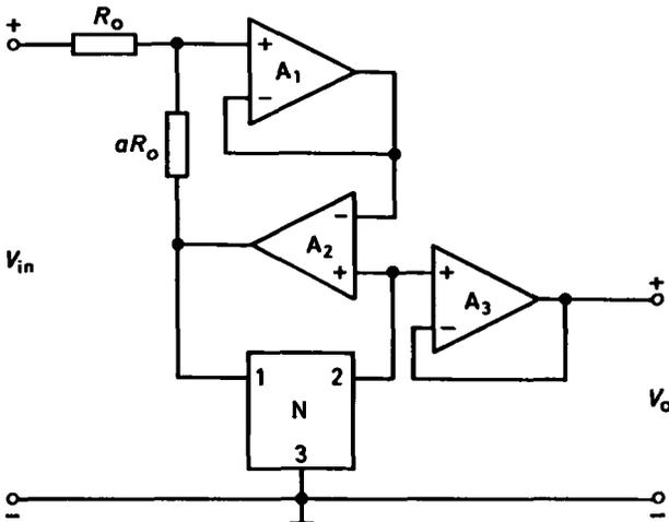
Fig. 2: The new active compensated canonic bandpass filter
