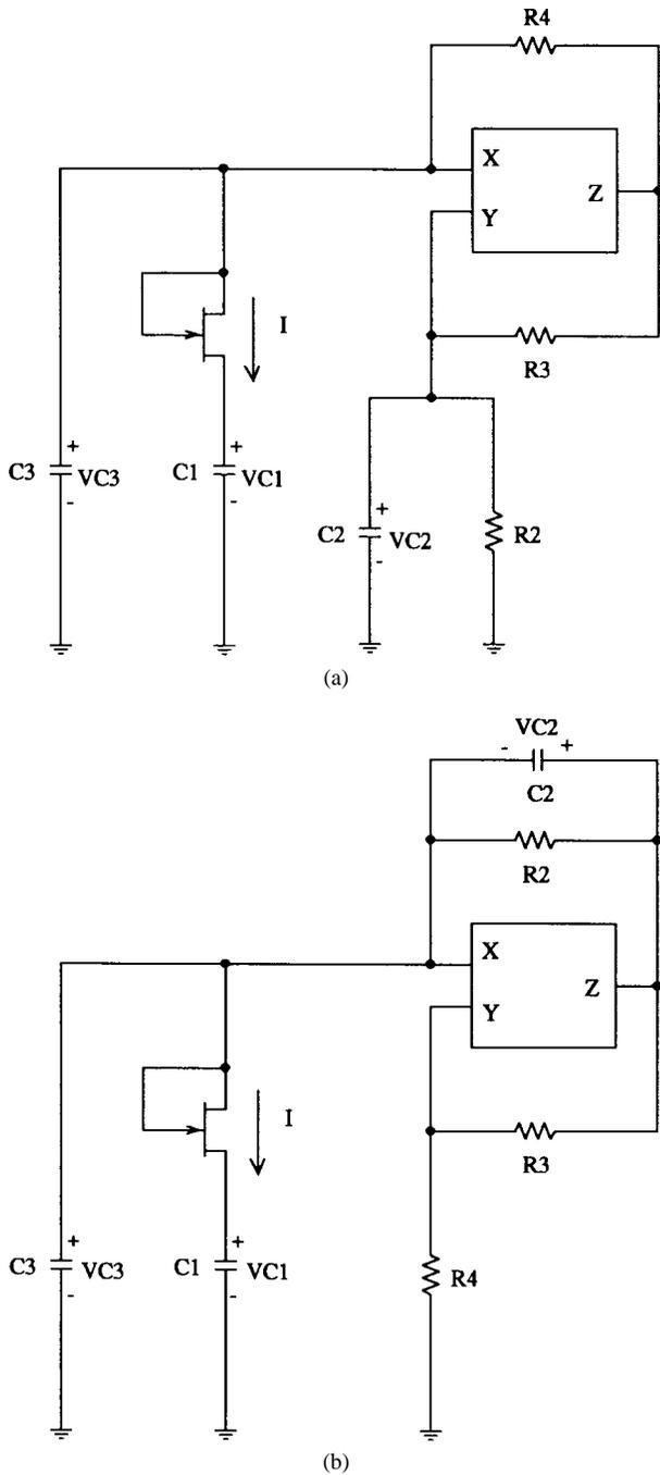
Fig. 1. The two proposed chaos generators using a single CCII.
