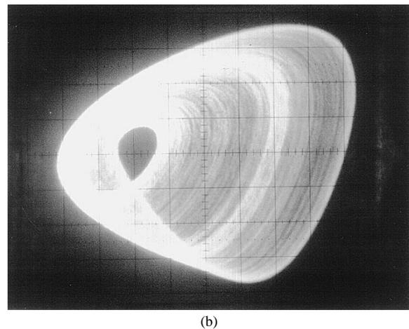
Fig. 4. (a) Numerical simulation of (6) given for  $\alpha = 2.67$ ,  $a = 18.84$ ,  $b = 20.4$ ,  $c = 0.2$ ,  $d = 16.12$ , and  $e = 16.3$ . (b) An experimental  $V_{C_1}$ – $V_{C_2}$  trajectory from the first chaos generator.
