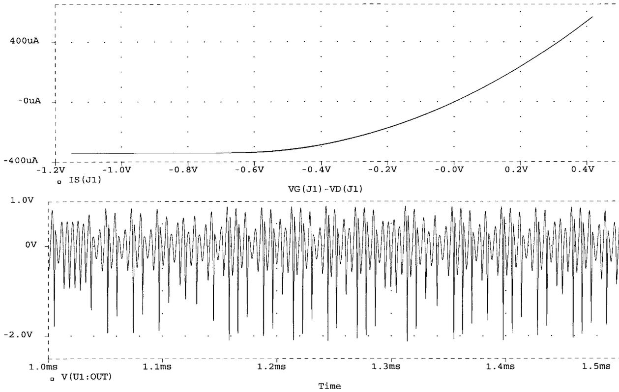
Fig. 2. The JFET characteristics and a sample of the output waveform of the first chaos generator obtained with  $R_2 = 2 \text{ K}\Omega$ ,  $R_3 = 500 \text{ }\Omega$ ,  $R_4 = 1090 \text{ }\Omega$ ,  $C_1 = C_3 = 2 \text{ nF}$ , and  $C_2 = 1 \text{ nF}$ .
