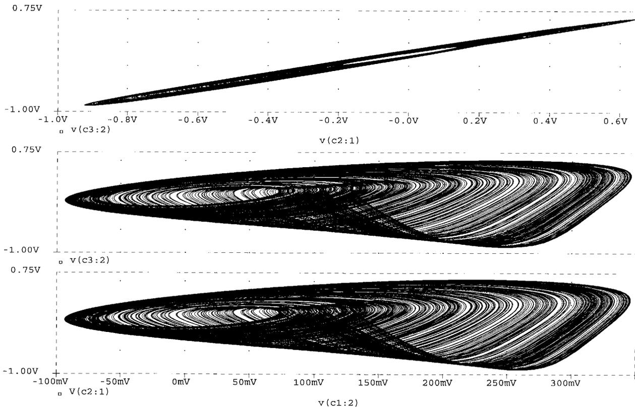
Fig. 3. The observed phase space trajectories of the first chaos generator obtained with  $R_2 = 2 \text{ K}\Omega$ ,  $R_3 = 500 \text{ }\Omega$ ,  $R_4 = 1090 \text{ }\Omega$ ,  $C_1 = C_3 = 2 \text{ nF}$ , and  $C_2 = 1 \text{ nF}$ .
