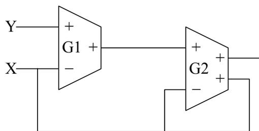
Fig. 4: Block diagram of the circuit shown in Fig. 3
