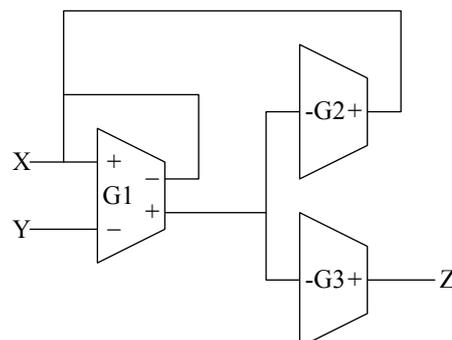
Fig. 8: Block diagram of the circuit shown in Fig. 7
