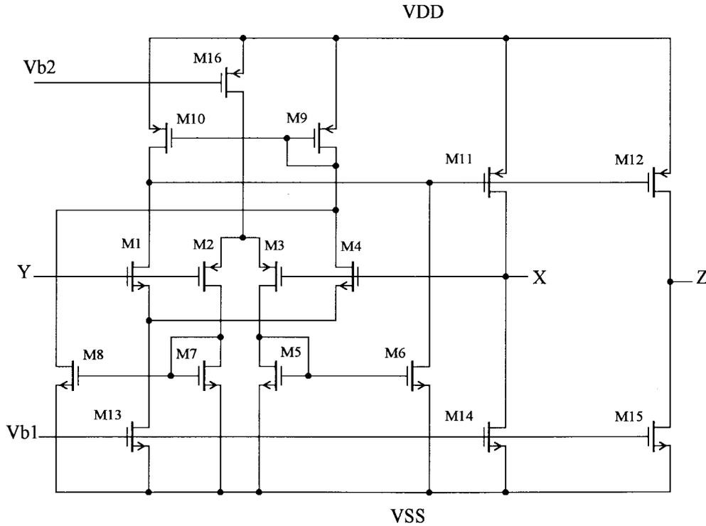
Fig. 1. The class A current conveyor circuit.
