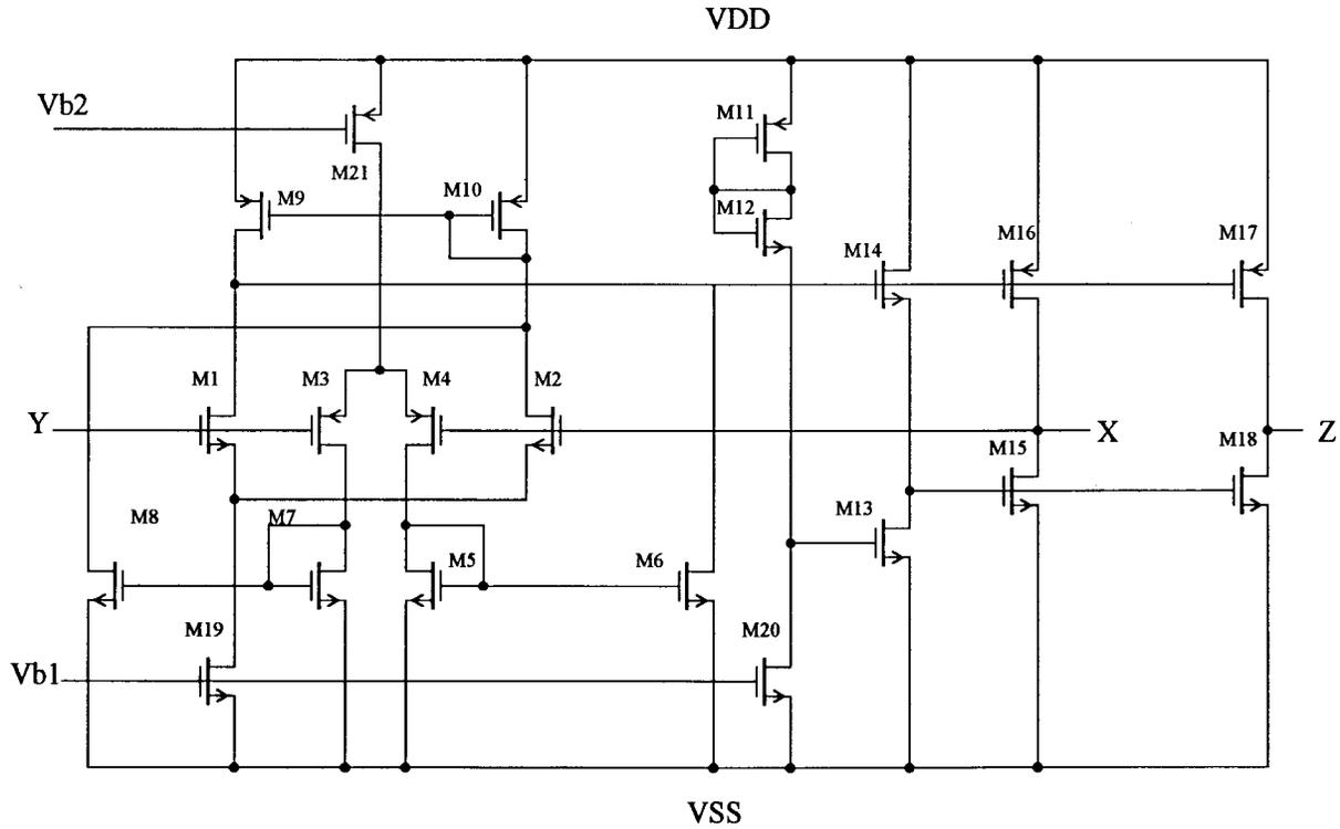
Fig. 3. The class AB current conveyor circuit.
