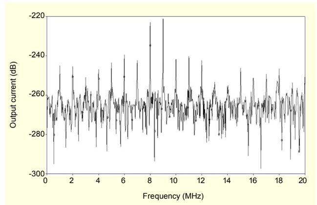
Fig. 12. The simulated IM3 frequency spectrum of the proposed Gm-C output current at input frequencies of 8 and 9 MHz.
