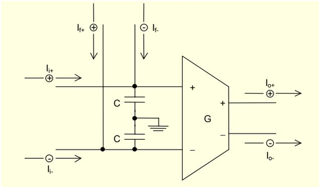
Fig. 9. The symbol of the differential current integrator.
