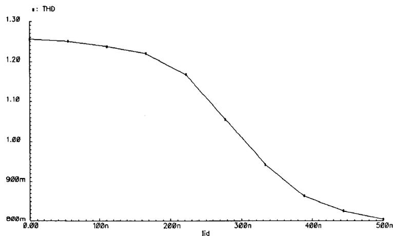
Fig. 17: THD versus the amplitude of the sinusoidal input current
