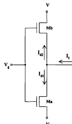
Fig. 4: The basic principle of current division
