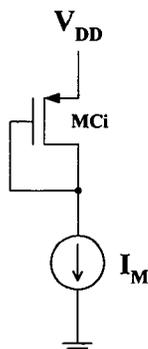
Fig. 9: The biasing circuit of the proposed transconductor
