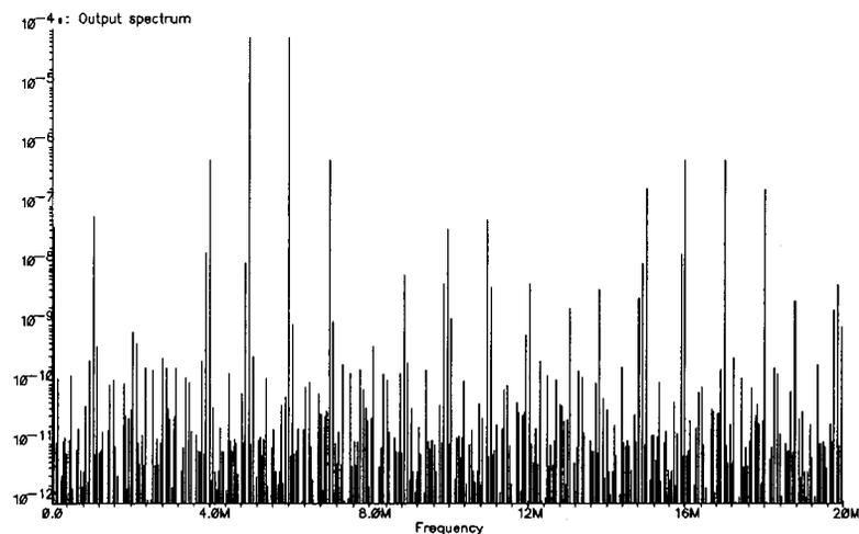
Fig. 15: IMD with a 5 MHz and 6 MHz input with 0.5  $\mu$ A amplitude each
