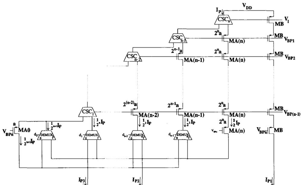
Fig. 7: The P part of the proposed digitally controlled transconductor
