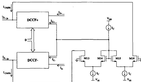
Fig. 10: The fully differential DCCF (FDDCCF)
