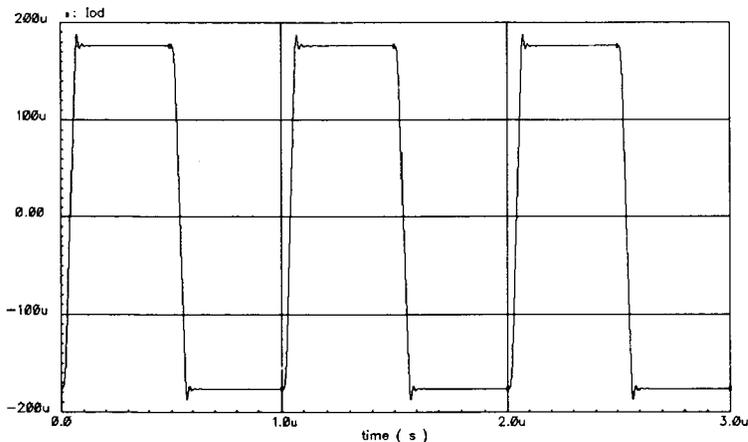
Fig. 16: Step response of the VGA
