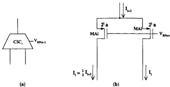
Fig. 6: The current steering cell (CSC)
