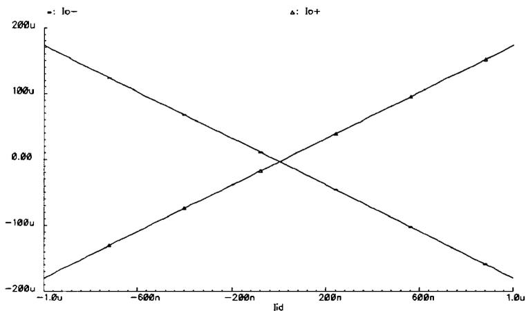
Fig. 13: The balanced output currents versus the differential input current (gain 50.7 dB)
