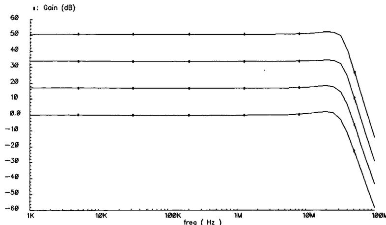
Fig. 14: Frequency response of the VGA (gain 50.7 dB)
