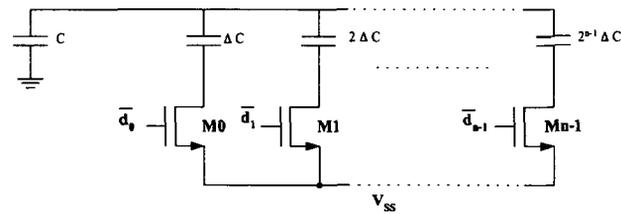
Fig. 12: The digitally controlled compensation capacitor
