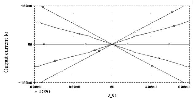
Fig. 8: The I-V characteristics for the four-quadrant multiplier circuit
