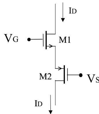
Fig. 1: The composite transistor proposed in [1, 2]
