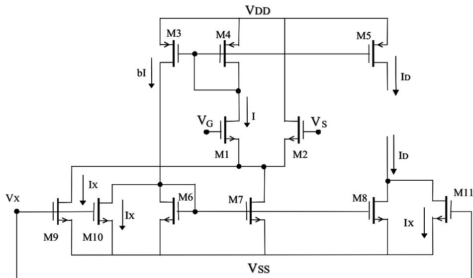
Fig. 3: The proposed composite transistor (CT)
