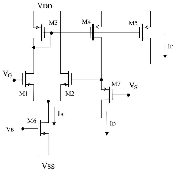
Fig. 2: The low voltage composite transistor proposed in [3, 4]
