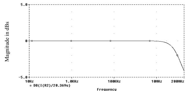
Fig. 10: The frequency characteristics for the four-quadrant multiplier circuit
