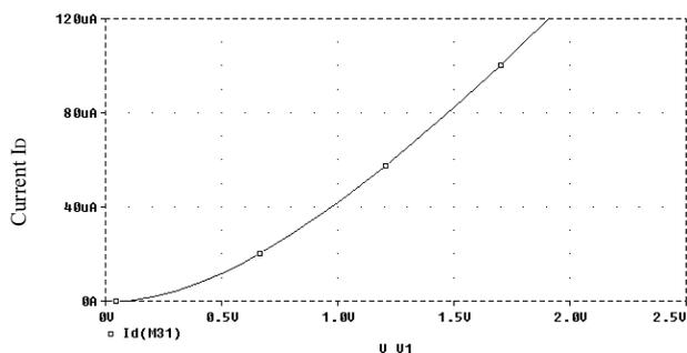
4 Fig. 7: The I-V characteristics for the composite transistor
