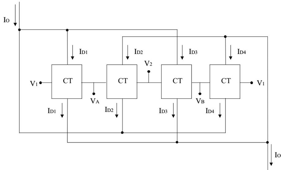
Fig. 6: The equivalent circuit of the CT taking in consideration the effect of mobility reduction
