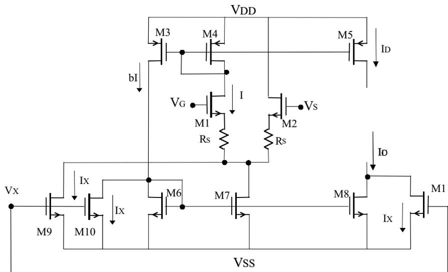
Fig. 5: The analog four-quadrant multiplier circuit using CT cells
