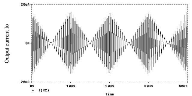
Fig. 9: The transient response of the output current of the multiplier circuit resulting from the multiplication of two differential input voltages
