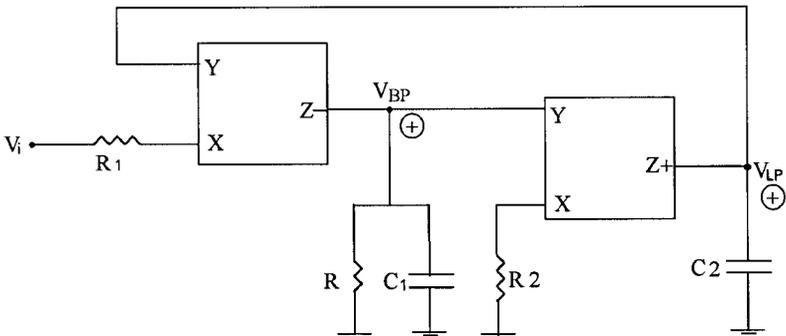
Figure 9. A grounded-C bandpass-lowpass filter using two opposite polarity CCII's.
