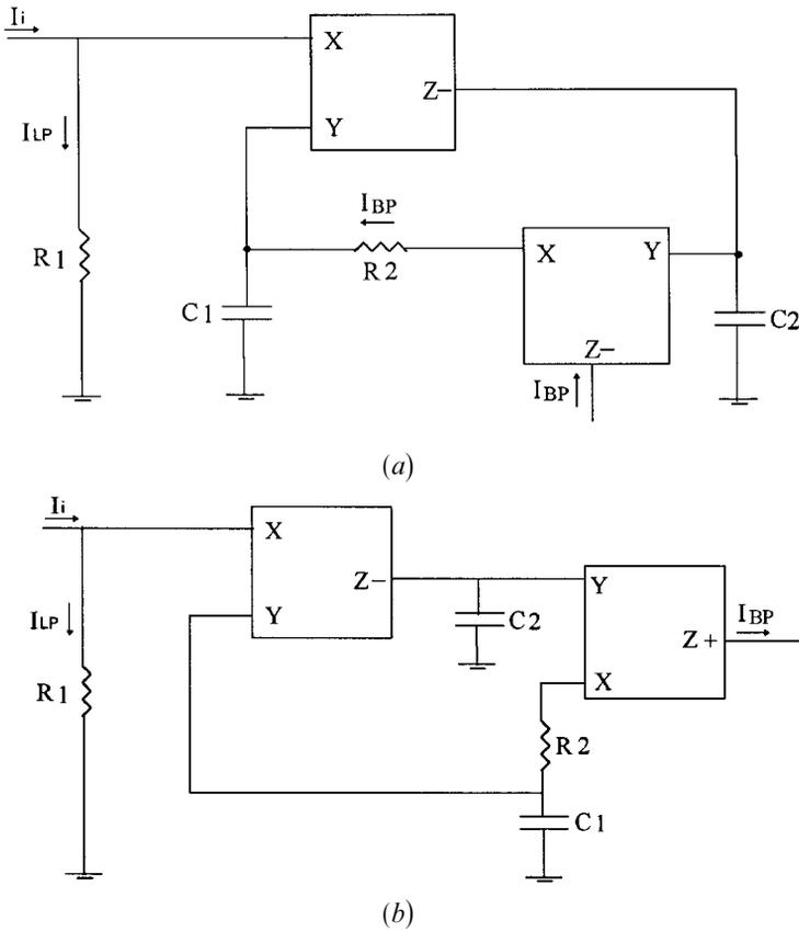
Figure 6. Current-mode grounded-C bandpass filters.
