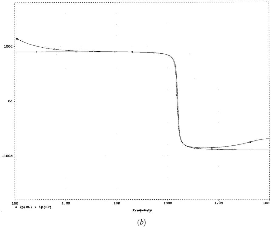
Figure 19. The magnitude and phase characteristics of the compensated current-mode bandpass filter of figure 6(b).
