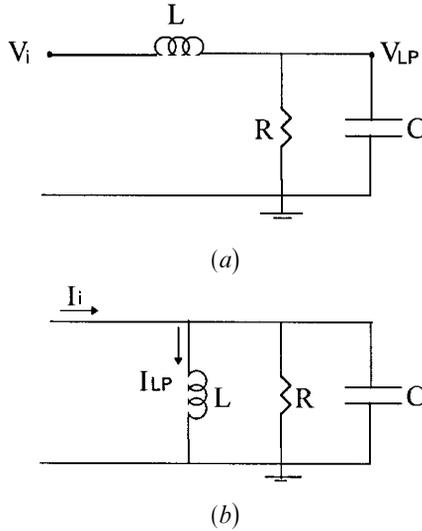
Figure 1. (a) Voltage-mode passive  $RLC$  lowpass filter; (b) current-mode passive  $RLC$  lowpass filter.
