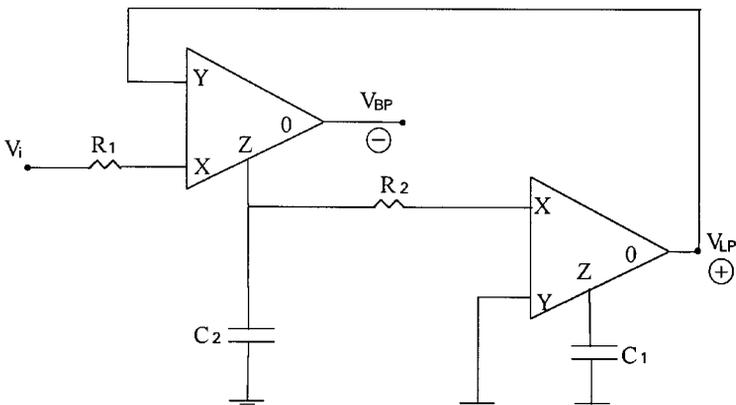
Figure 4. New inverting bandpass, non-inverting lowpass filter using CFOAs.
