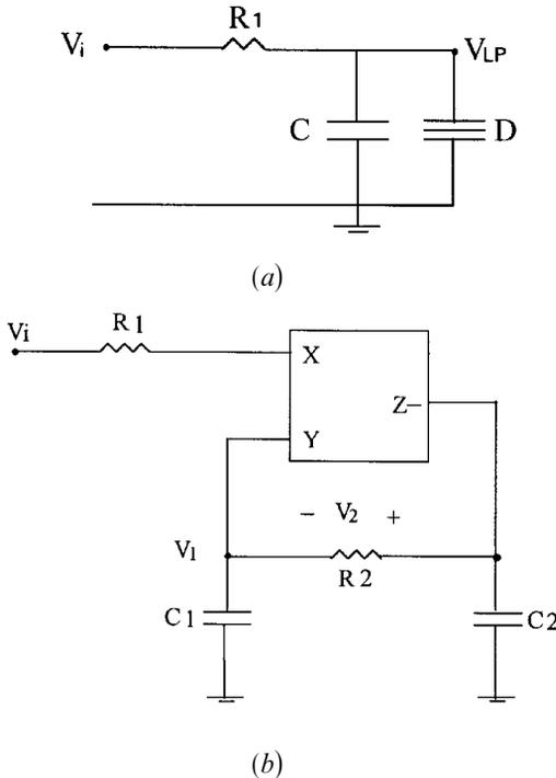
Figure 2. (a) Voltage-mode active  $RCD$  lowpass filter; (b) voltage-mode grounded- $C$  lowpass filter using CCII-.
