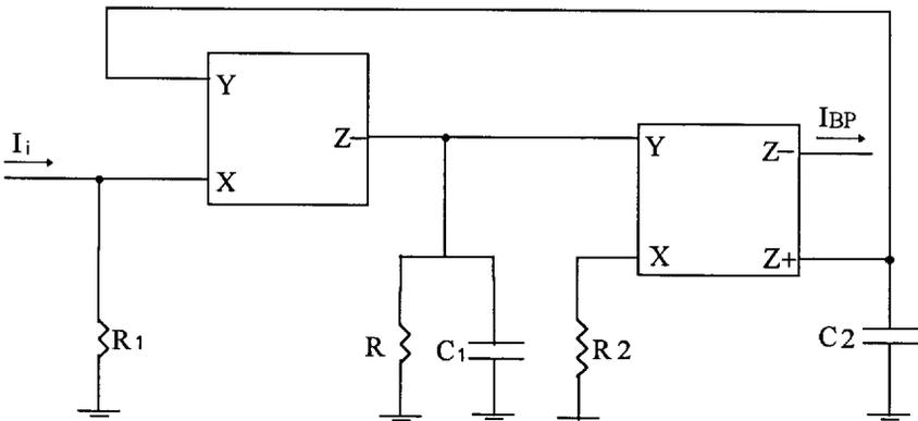
Figure 11. A grounded- $R$  grounded- $C$  current-mode bandpass filter.
