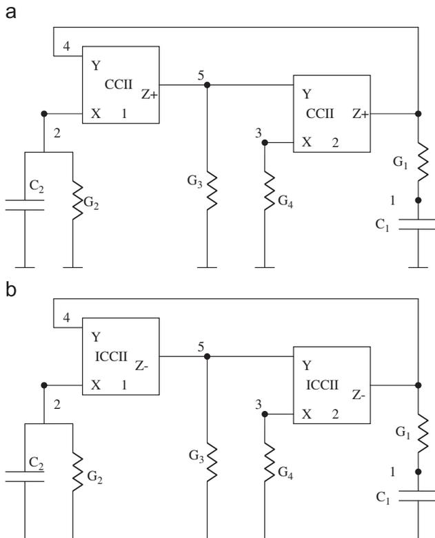
Fig. 5. (a) Realization of class II type A circuit from Fig. 2(a) and (b) realization of class II type B circuit from Fig. 3(a).
