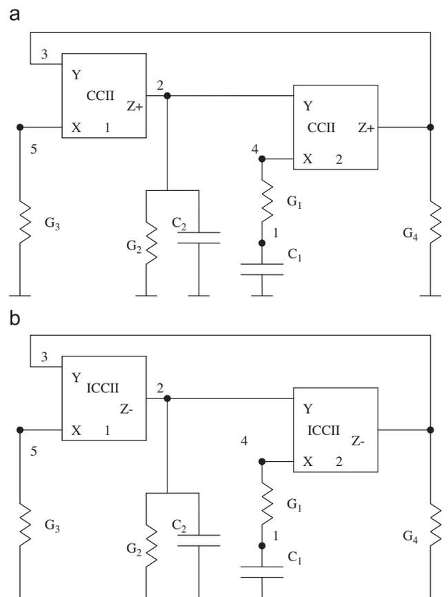
Fig. 4. (a) Realization of class-I type A circuit from Fig. 2(a) and (b) realization of class I type B circuit from Fig. 3(a).
