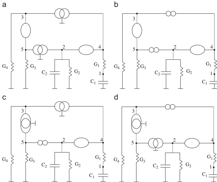
Fig. 2. Four alternative realizations of type A oscillators: (a) realization A-1, (b) realization A-2, (c) realization A-3, and (d) realization A-4.
