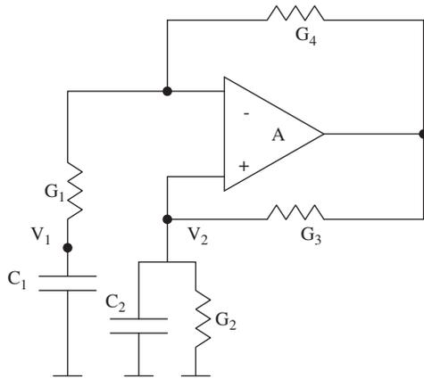
Fig. 1. Grounded capacitor Wien oscillator using Op Amp.
