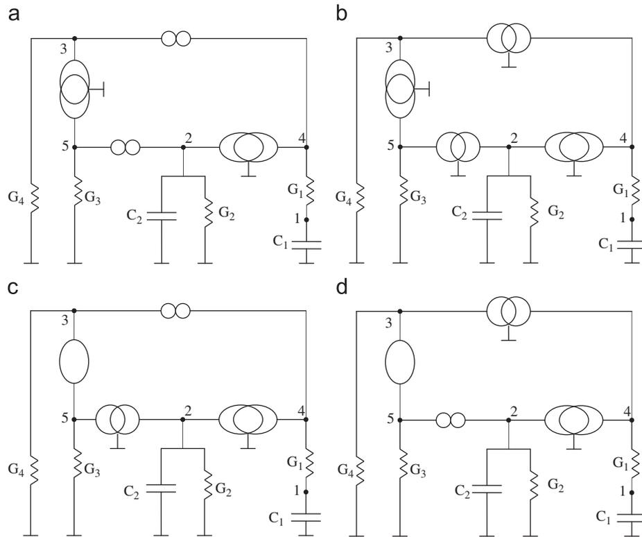
Fig. 3. Four alternative realizations of type B oscillators: (a) realization B-1, (b) realization B-2, (c) realization B-3, and (d) realization B-4.
