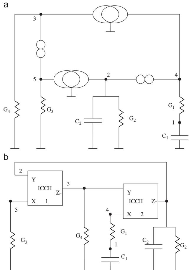
Fig. 6. (a) Adjoint circuit to the circuit of Fig. 2(a) and (b) realization of class III type A circuit from Fig. 6(a).
