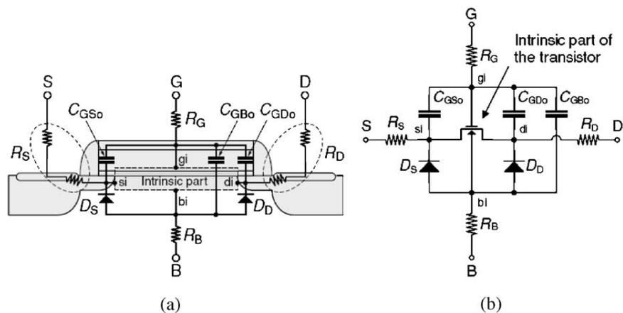
Fig. 2. (a) Definition of the extrinsic part of the MOS transistor and the extrinsic components including the series access resistances, the overlap parasitic capacitances, and the junction parasitic capacitances. (b) Simple equivalent circuit of the extrinsic part corresponding to (a) [13,14].
