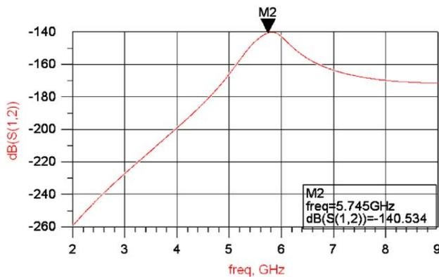
Fig. 5. Simulated reverse isolation of the LNA.
