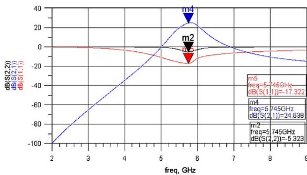
Fig. 4. Simulated input return loss, LNA gain, and output return loss of the LNA.
