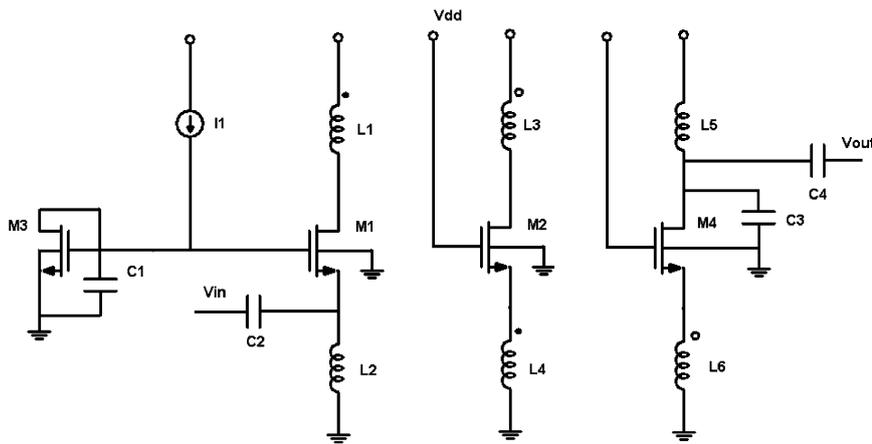
Fig. 3. Three stages low noise amplifier.
