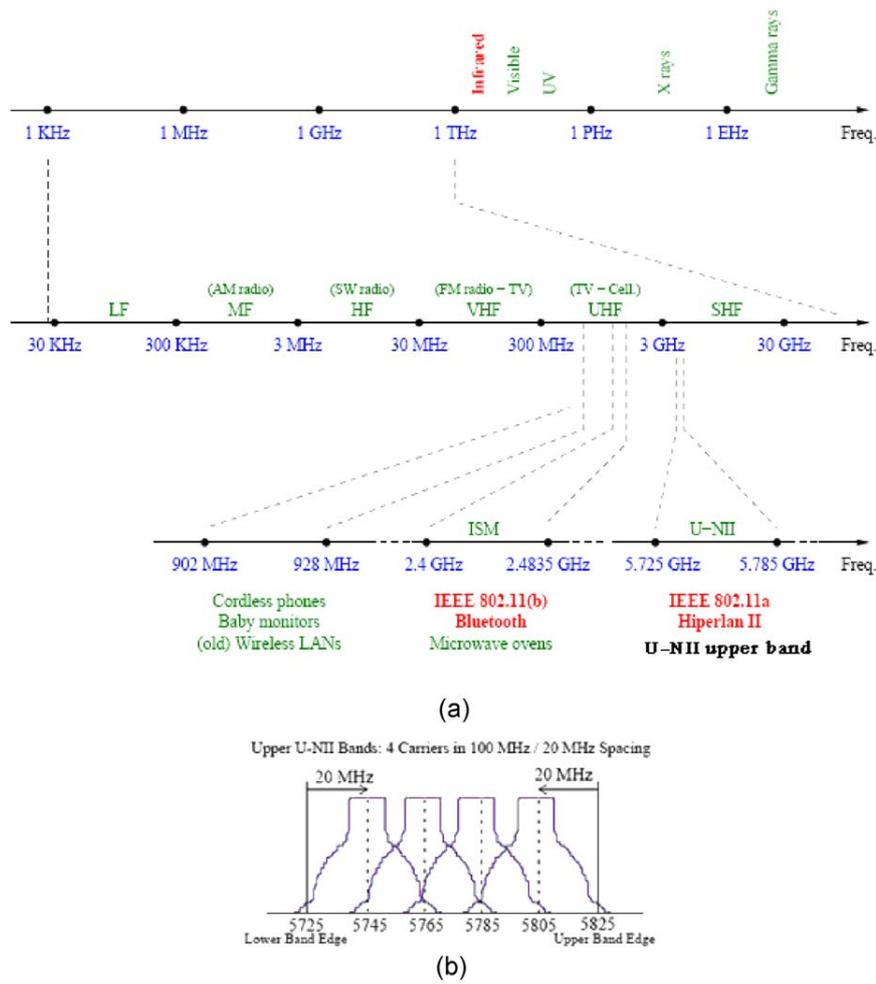
Fig. 1. (a) The EM spectrum allocation. (b) OFDM Phy frequency channel plan for the US [2,8–11].
