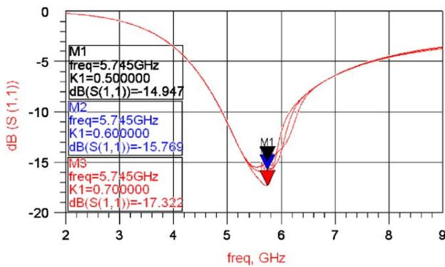
Fig. 7. Simulated input return loss of the LNA.
