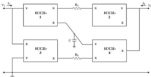
Fig. 10 Proposed ICCII– based floating inductor
