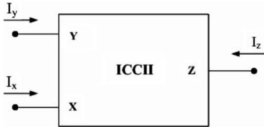
Fig. 1 Block diagram of ICCII
