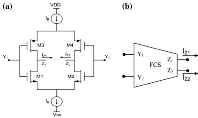
**Fig. 5** (a) The CMOS FCS circuit [8] (b) A proposed symbolic representation of the FCS
