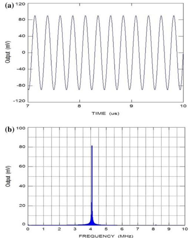
**Fig. 9** (a) The output waveform of the proposed oscillator (b) The corresponding Fourier transform
