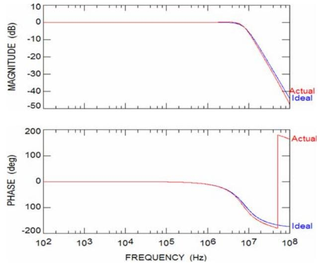
Fig. 12 AC response of the low pass filter using the proposed inductor compared with the ideal curves
