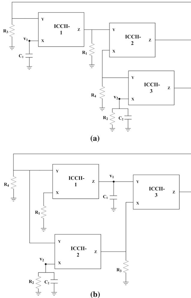
**Fig. 8** (a) The first proposed oscillator topology (b) The second oscillator topology
