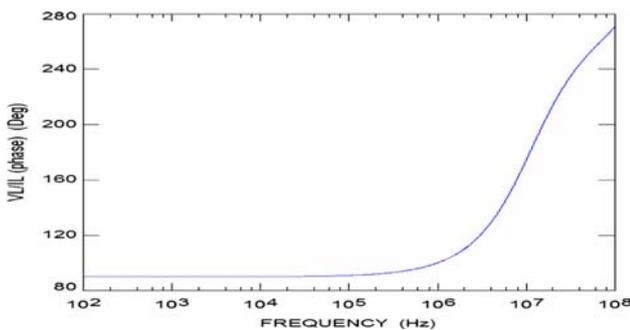
Fig. 11 The phase of the input impedance of the proposed inductor
