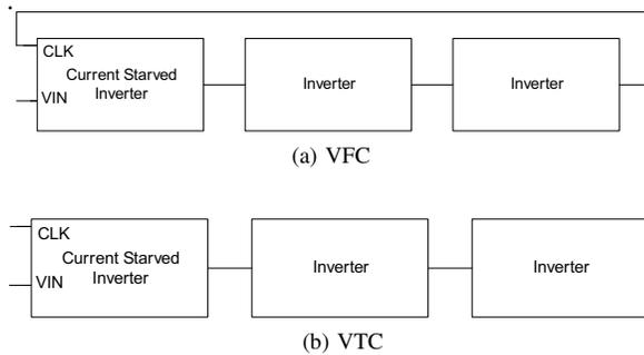
Fig. 1. VFC and VTC circuits block diagram
