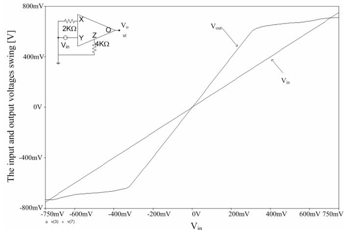
Figure 4. The input and output voltage swing for CFOA-based amplifier.
