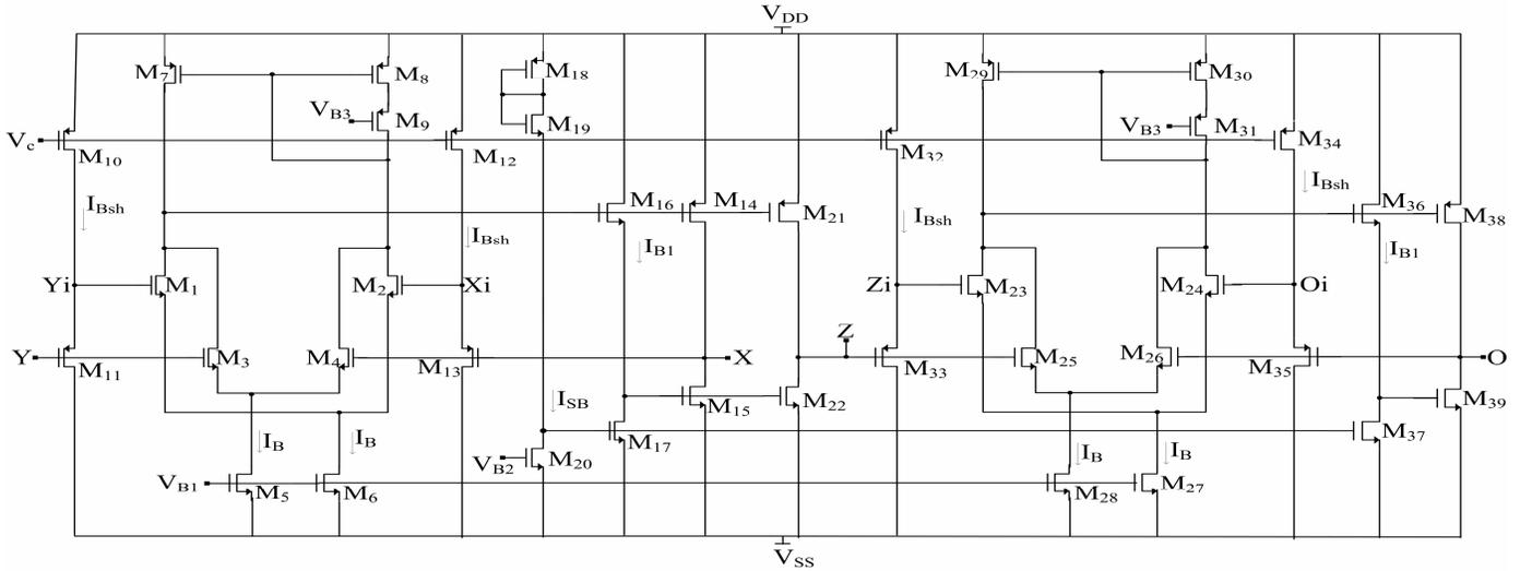
Figure 2. CMOS realization of the proposed CFOA.
