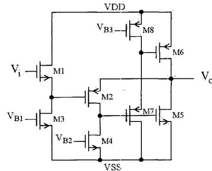
Figure 1. The uncompensated voltage buffer.
