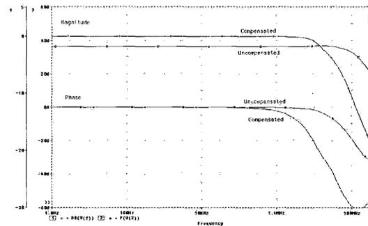
**Figure 4.** The magnitude and phase responses of the buffer circuits of Figs. 1 and 2.
