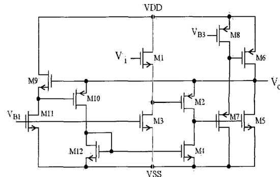
Figure 2. The compensated buffer circuit.
