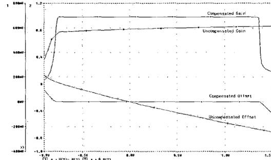
**Figure 3.** The voltage transfer gain and the voltage offset variations with respect to the input voltage for the buffer circuits of Figs. 1 and 2.
