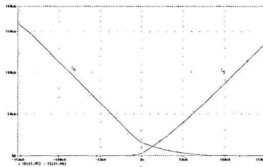
**Figure 6.** The push-pull action provided by the output stage of the buffer circuit of Fig.2.
