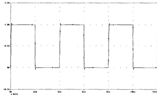
**Figure 5.** Transient response of the buffer circuit of Fig.2.
