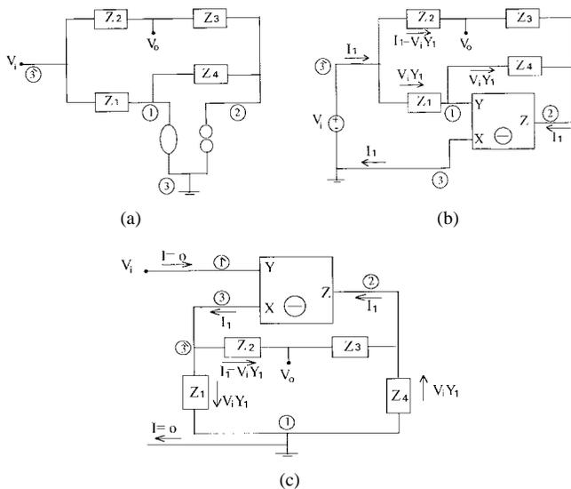
Fig. 3. (a) The nullor equivalent circuit to that Fig. 1(b). (b) The theoretical CC II equivalent circuit. (c) The practical CC II equivalent circuit [14].
