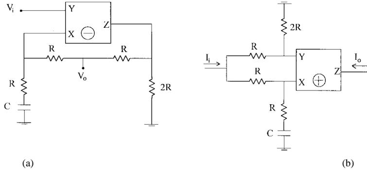
Fig. 5. (a) A new grounded  $C$  all-pass voltage mode circuit. (b) A new grounded  $C$  all-pass current mode circuit.
