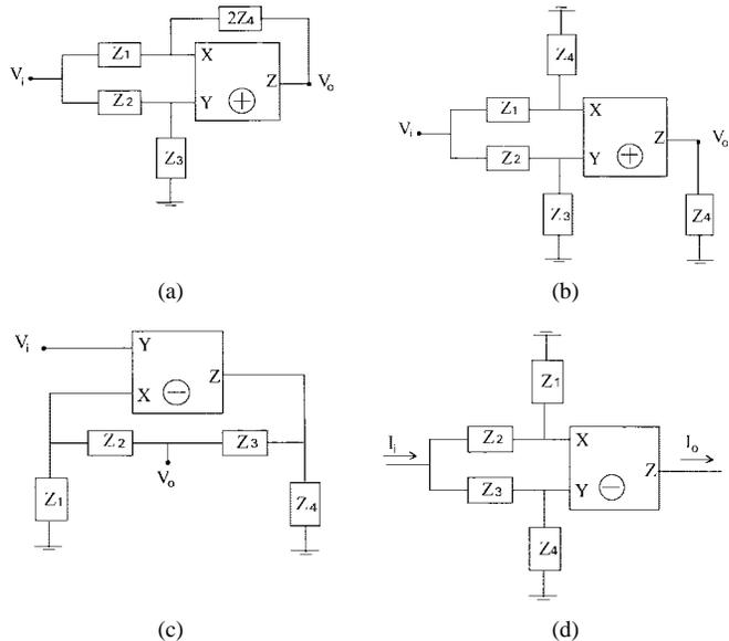
Fig. 2. (a) The CC II(+) all-pass circuit [6], (b) an equivalent CC II(+) all-pass circuit [15], (c) the CC II(-) all-pass voltage mode circuit [14], and (d) the CC II(-) all-pass current mode circuit [10].
