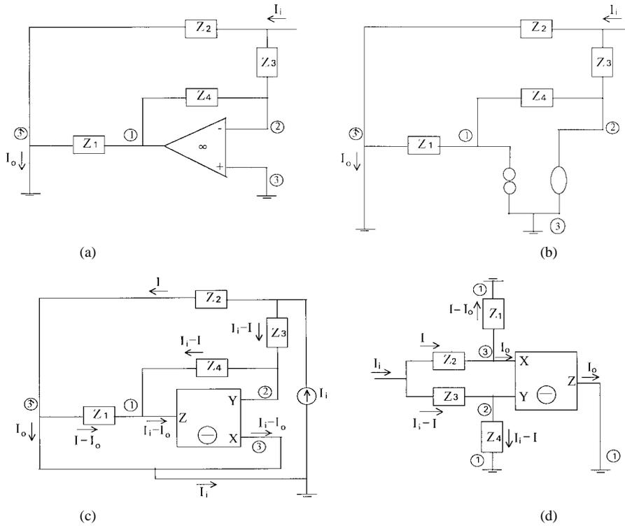
Fig. 4. (a) The adjoint current mode circuit obtained from Fig. 1(b). (b) The nullor equivalent circuit. (c) The theoretical CC II equivalent circuit. (d) The current mode CC II circuit [10].
