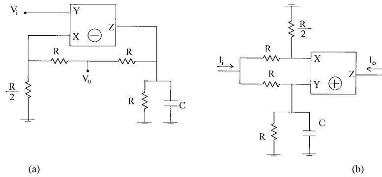
Fig. 6. (a) Another new grounded  $C$  all-pass voltage mode circuit. (b) Another new grounded  $C$  all-pass current mode circuit.
