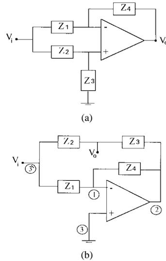
Fig. 1. (a) The differential input op amp circuit [1] and (b) the single input op amp circuit [2], [3].
