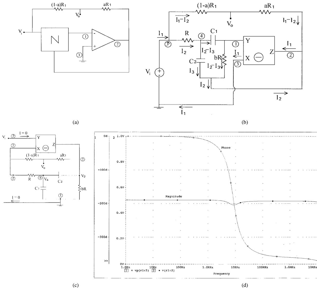
Fig. 7. (a) The generalized all-pass filter using the single input op amp, (b) the theoretical CC II equivalent circuit, (c) the new generalized biquad circuit using a CC II(-), and (d) simulation results for the circuit of (c) with  $V_i = 1$  V.
