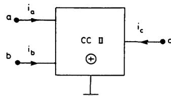
Fig. 1 Symbolic representation of the second-generation current conveyor
