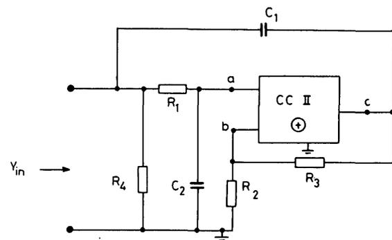
Fig. 2 New canonic circuit realising an ideal f.d.n.r., a lossy f.d.n.r., a parallel-tuned circuit and an oscillator
