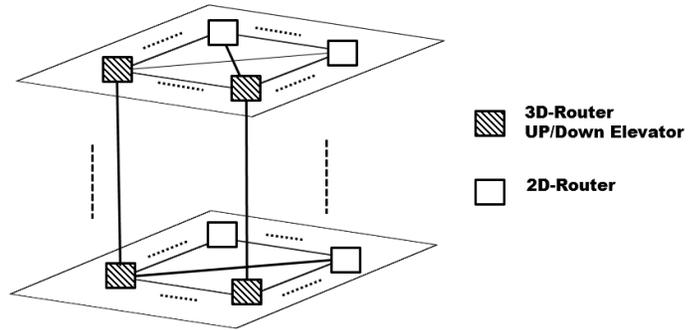
Fig. 2: The 3D-NoC in 2D Mesh Topology
