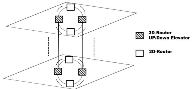
Fig. 3: The 3D-NoC in 2D Ring Topology
