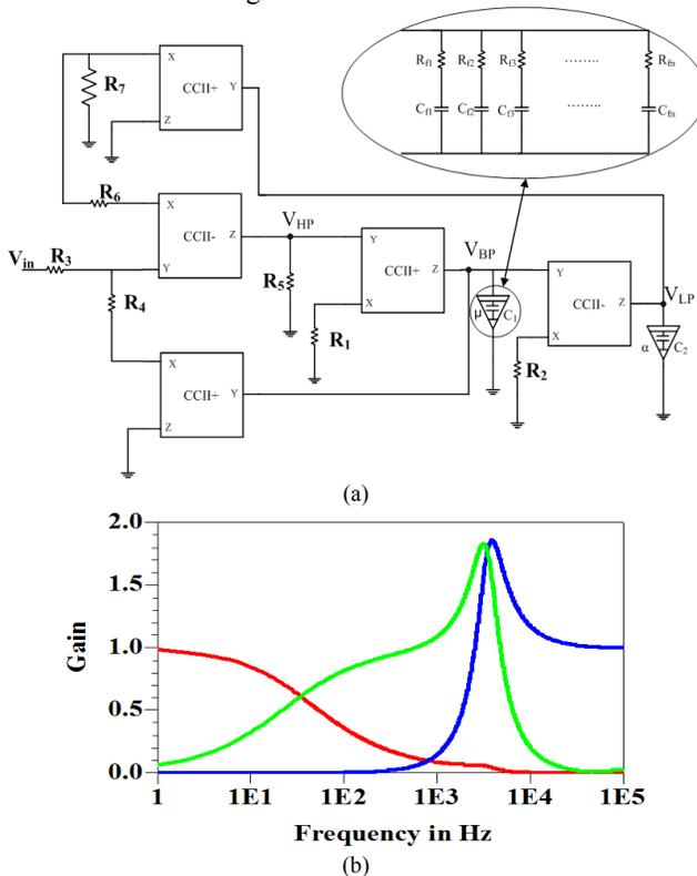
Figure 6. (a) CCII-based fractional order KHN filter, and (b) circuit simulation for  $(\alpha, \beta) = (1.5, 2.25)$ .
