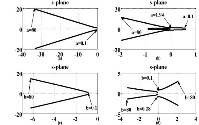
Figure 1. Movement of the poles with respect to  $a$  and  $b$ , (a)  $\alpha = 0.4, \beta = 1.6, b = 1$ , (b)  $\alpha = 1.6, \beta = 3.4, b = 1$ , (c)  $\alpha = 0.4, \beta = 1.6, a = 1$ , and (d)  $\alpha = 1.6, \beta = 3.4, a = 1$
