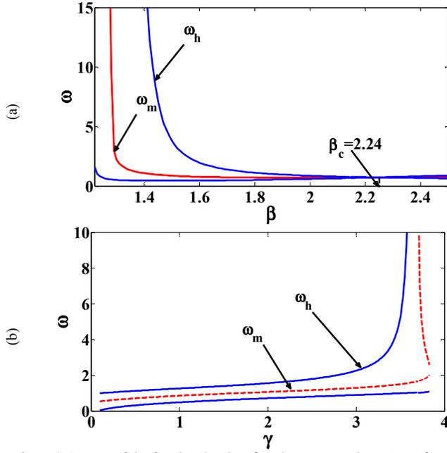
Figure 3. Impact of the fractional orders  $\beta$  and  $\gamma$  on  $\omega_m$  and  $\omega_h$  at  $a = b = d = 1$  and, (a)  $\alpha = 0.8\beta$  and  $\gamma = 1.2$ , and (b)  $\beta = 3.7$  and  $\alpha = 1.4$
