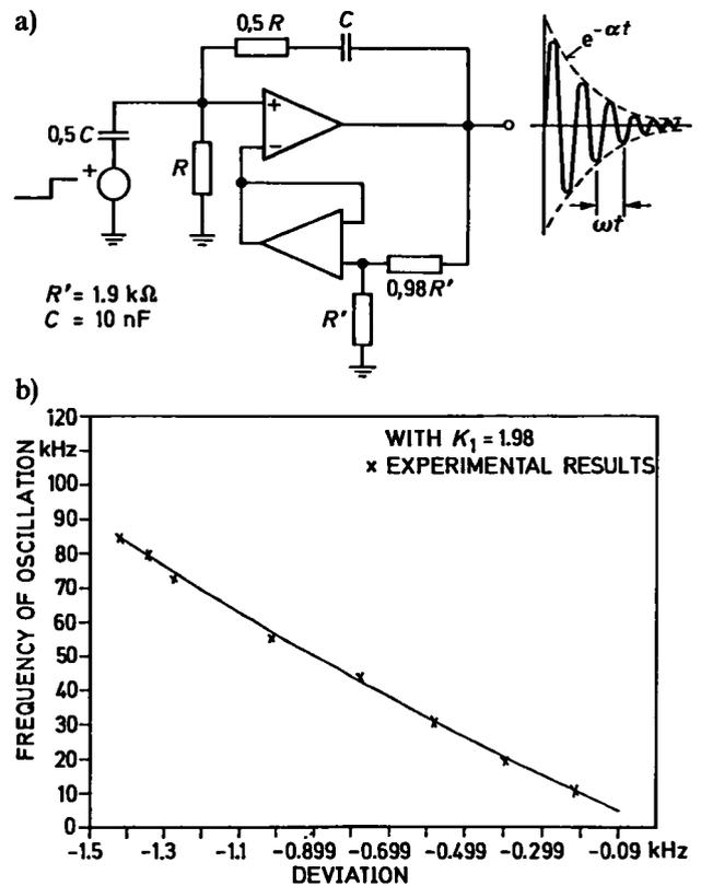
Fig. 13: Closed-loop test of the fourth realization
