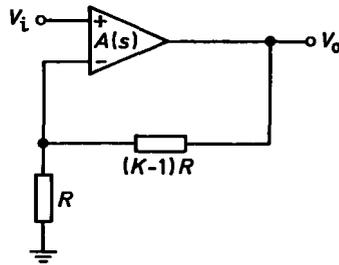
Fig. 2: The uncompensated amplifier
