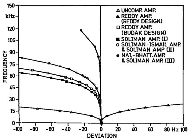
Fig. 3: Upper half-plane pole loci (Equal R, C design)
