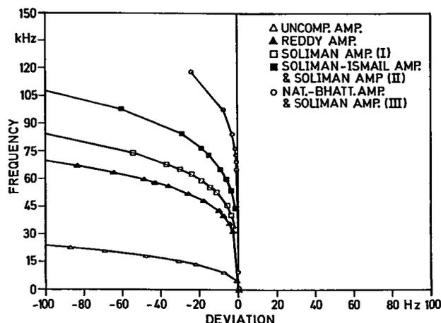
Fig. 4: Upper half-plane pole loci (The optimum design of the circuit of Fig. 1a)
