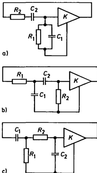
Fig. 1: Three types of oscillators
