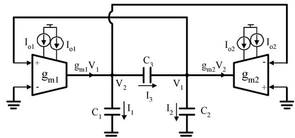
Fig. 5. The equivalent SRD counterpart of the example oscillator.
