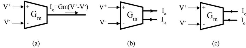
Fig. 1. Differential input linear transconductors. (a) Single output. (b) Double output. (c) Balanced output.
