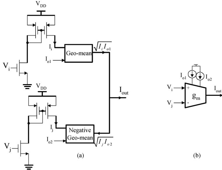
Fig. 2. (a) SRD equivalent implementation of single output linear transconductor. (b) Its symbol.
