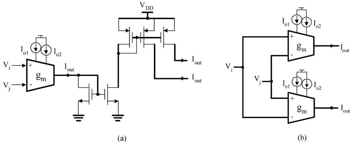
Fig. 3. (a) SRD equivalent implementation of double output linear transconductor. (b) SRD equivalent implementation of balanced output linear transconductor.
