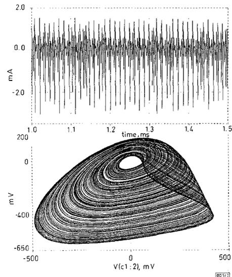
Fig. 2 PSPICE simulations of output current driving  $1k\Omega$  load and  $V_{C1}-V_{C2}$  phase space trajectory
