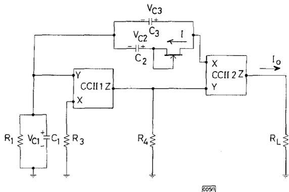
Fig. 1 Proposed current mode chaos generator
