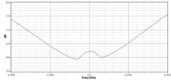
Figure 10 Simulated noise figure
