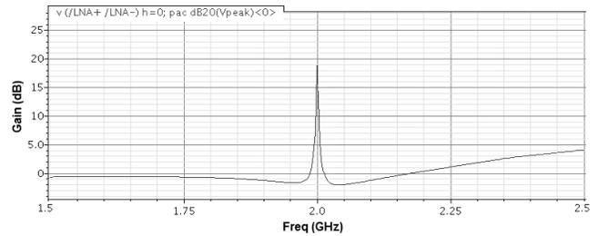
Figure 9 Simulated closed loop frequency response
