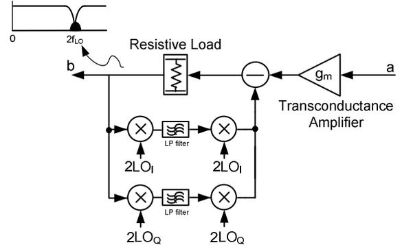
Figure 3 Implementation of the notch filter at  $2f_{LO}$
