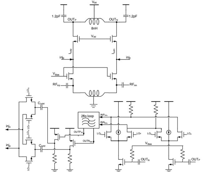
Figure 7 Circuit implementation of the main feedback loop (for clarity, only 1 branch is shown)
