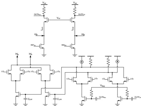
Figure 8 Circuit implementation of the  $2f_{LO}$  notch filter (1 branch only)
