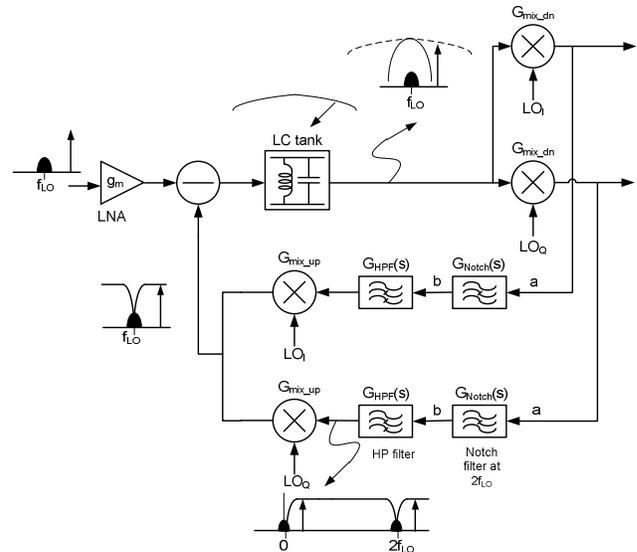
Figure 1 Proposed narrowband RF front-end architecture with  $2f_{LO}$  notch
