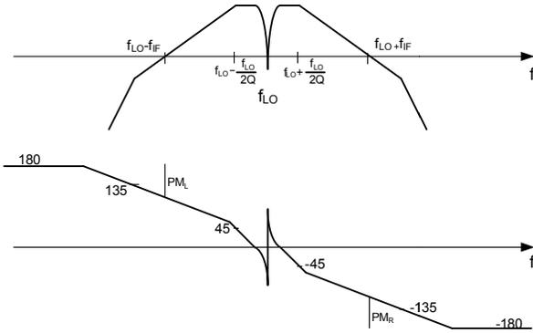
Figure 5 Bode plot of open loop gain
