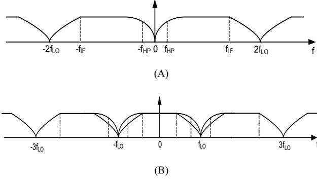
Figure 4 (A) Baseband filter response (B) RF notch filter response
