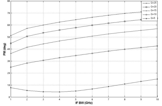
Figure 6 PM versus IF BW for different Q of LNA's LC tank
