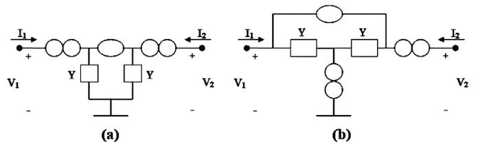
Fig. 11. (a) Current mirror representation using nullor elements and two equal passive elements. (b) Equivalent current mirror representation using nullor elements and two equal passive elements.
