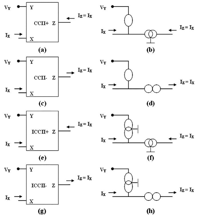
Fig. 6. (a) CCII+ symbol. (b) CCII+ nullor-mirror representation. (c) CCII- symbol. (d) CCII- nullor-mirror representation. (e) ICCII+ symbol. (f) ICCII+ nullor-mirror representation. (g) ICCII- symbol. (h) ICCII- nullor-mirror representation.
