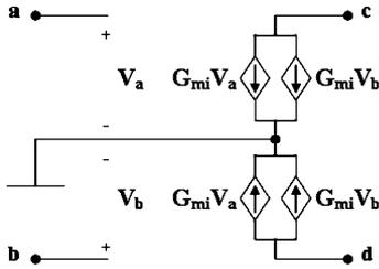
Fig. 5. Voltage controlled current sources based model for a mirror pair with a voltage mirror connected between nodes  $a$  and  $b$  and a current mirror connected between nodes  $c$  and  $d$ .
