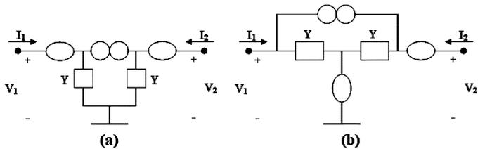
Fig. 10. (a) Voltage mirror representation using nullor elements and two equal passive elements. (b) Equivalent voltage mirror representation using nullor elements and two equal passive elements.
