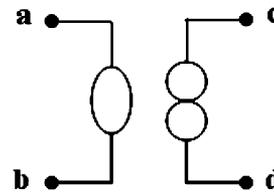
Fig. 2. Two-port nullor with a nullator connected between nodes a and b and a norator connected between nodes c and d.
