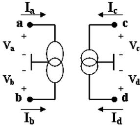
Fig. 4. Four-port mirror pair with a voltage mirror connected between nodes  $a$  and  $b$  and a current mirror connected between nodes  $c$  and  $d$ .
