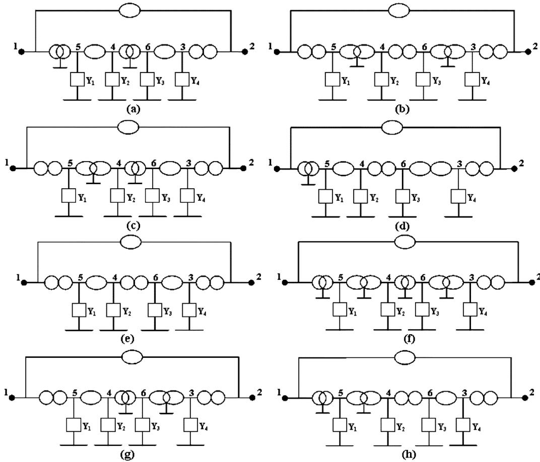
Fig. 9. Eight equivalent nullor-mirror descriptions for a GIC with three active devices and four grounded passive elements.
