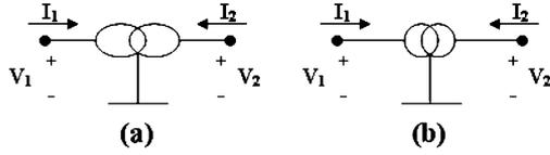
Fig. 3. Mirror elements. (a) Voltage mirror. (b) Current mirror.
