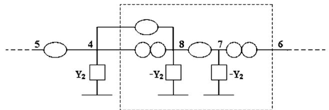
Fig. 12. Equivalent nullor circuit for the current mirror connected between nodes 4 and 6 in the GIC described in (31).
