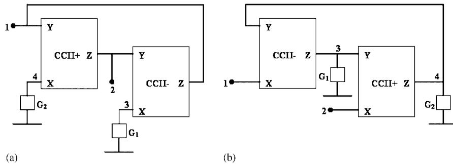
Figure 6. CCII-based gyrators with two different CCIIs and two grounded conductances: (a) Y–Z input/output terminals and (b) X input/output terminals.
