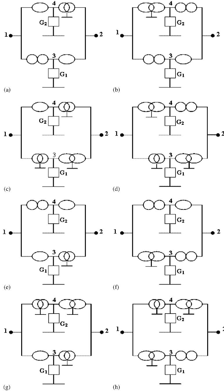
Figure 3. Gyrator nullor-mirror representations with two different pairs of pathological elements and two grounded conductances.
