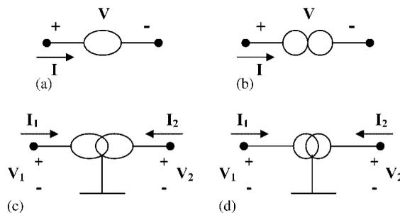
Figure 1. Nullor–mirror elements: (a) nullator; (b) norator; (c) voltage mirror; and (d) current mirror.
