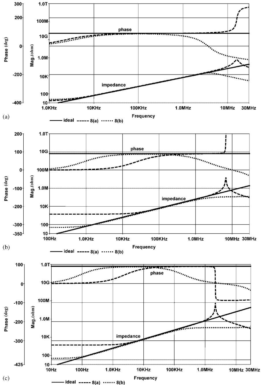
Figure 13. Magnitude and phase responses for the impedance of the simulated grounded inductances in Figure 8 and ideal inductance: (a) 1 mH; (b) 10 mH; and (c) 100 mH.
