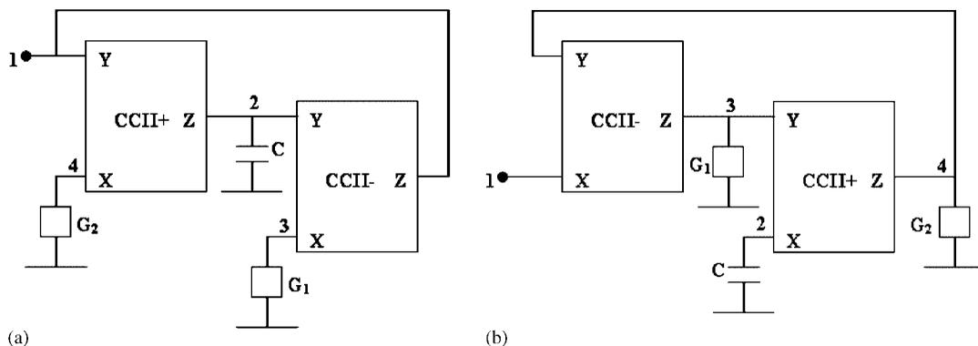
Figure 8. Simulated grounded coils using the CCII-based gyrators in Figure 6.
