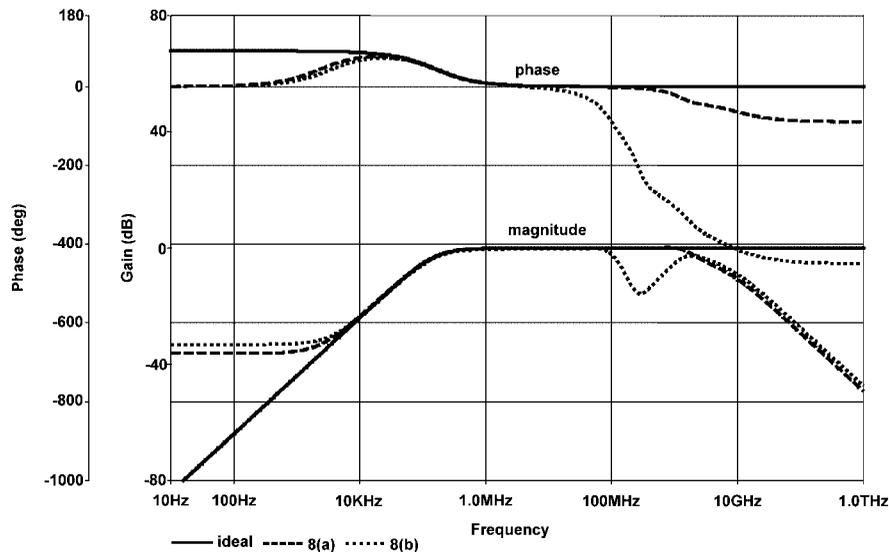
Figure 15. Magnitude and phase responses for the gain of the high-pass  $RL$  section in Figure 14 constructed using the simulated grounded inductances in Figure 8 and ideal inductance.
