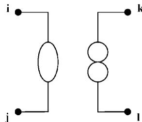
Figure 2. Nullor with a nullator connected between nodes  $i$  and  $j$  and a norator connected between nodes  $k$  and  $l$ .
