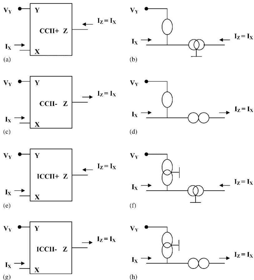
Figure 5. (a) The CCII+ symbol, (b) the CCII+ nullor-mirror representation, (c) the CCII- symbol, (d) the CCII- nullor-mirror representation, (e) the ICCII+ symbol, (f) the ICCII+ nullor-mirror representation, (g) the ICCII- symbol, and (h) the ICCII- nullor-mirror representation.
