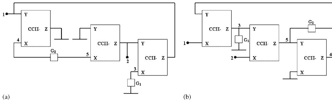
Figure 7. CCII-based gyrators with three similar CCIIs; one grounded conductance and one floating conductance: (a) Y–Z input/output terminals and (b) X input/output terminals.
