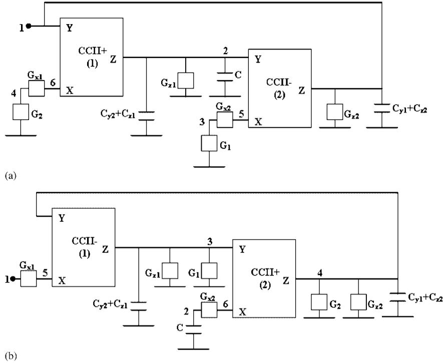
Figure 10. Circuit representation for the simulated grounded coils in Figure 8, including the CCII's associated parasitic elements.
