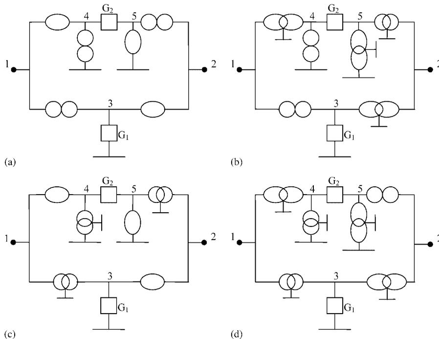
Figure 4. Gyrator nullor–mirror representations with three identical pairs of pathological elements; one grounded conductance and one floating conductance.
