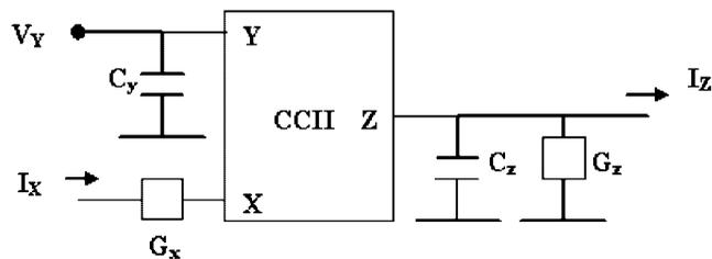
Figure 9. CCII symbolic representation including a modeling for the parasitic impedance components at the CCII terminals.
