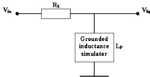
Figure 14. High-pass  $RL$  section with a floating resistance  $R_S$  and a grounded inductance simulator  $L_P$ .
