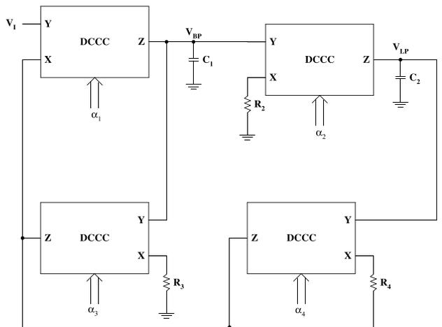
Fig. 16. The proposed digitally tuned filter.
