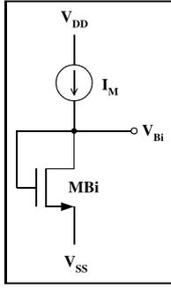
Fig. 6. The biasing circuit of the CDC cell.
