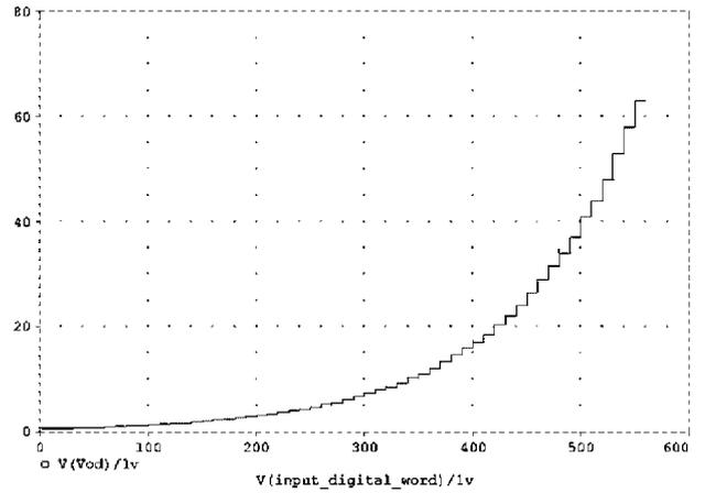
Fig. 12. Gain of the fully differential VGA versus input digital control word.
