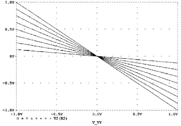
Fig. 8. Z terminal voltage for different values of  $\alpha$  when  $R_x = R_z = 10$  k $\Omega$ .
