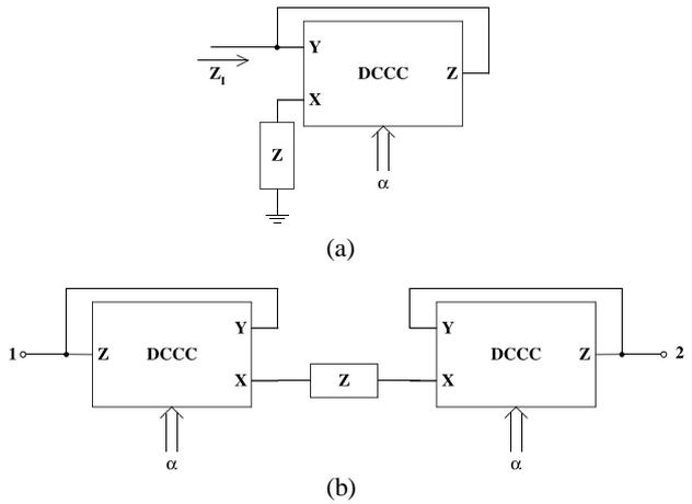
Fig. 15. Another realization of DCIC (a) Grounded DCIC (b) Floating DCIC.
