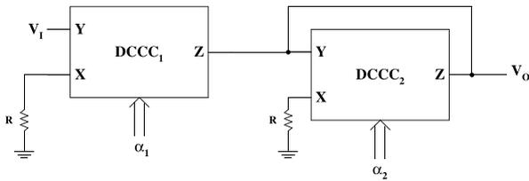
Fig. 10. The proposed digitally controlled VGA.
