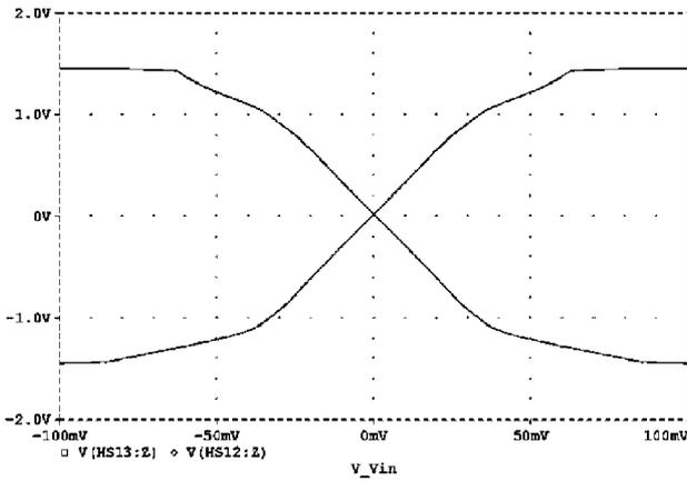
Fig. 13. The balanced output of the differential VGA versus the differential input at the maximum gain (36 dB).
