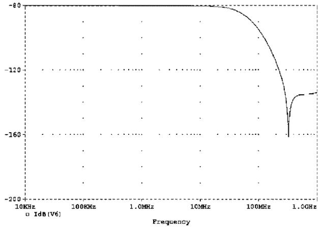
Fig. 9. Frequency response of the Z terminal current when  $R_x = 10$  k $\Omega$ .
