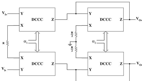
Fig. 11. Fully differential digitally controlled VGA.
