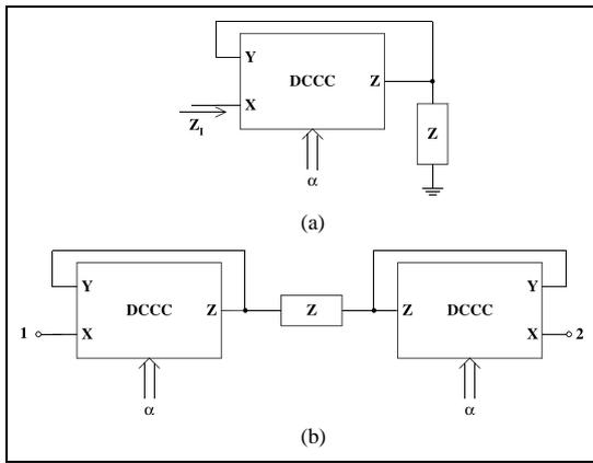
Fig. 14. Realization of DCIC (a) Grounded DCIC (b) Floating DCIC.
