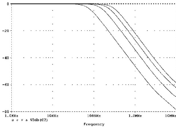
Fig. 18. Lowpass frequency responses for different cut-off frequencies.
