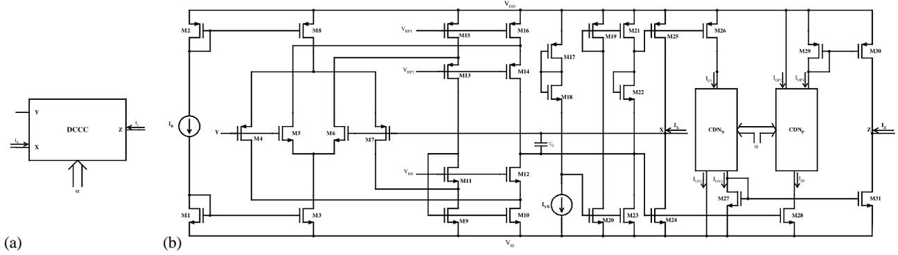
Fig. 1. The DCCC (a) symbol (b) circuit realization.
