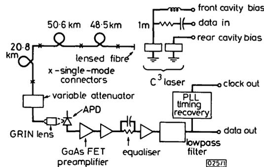
Fig. 1 Block diagram of 1 Gbit/s 120 km experiment described in the text
