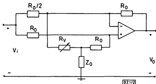
Fig. 2 Proposed variable equaliser with  $K = 2$
