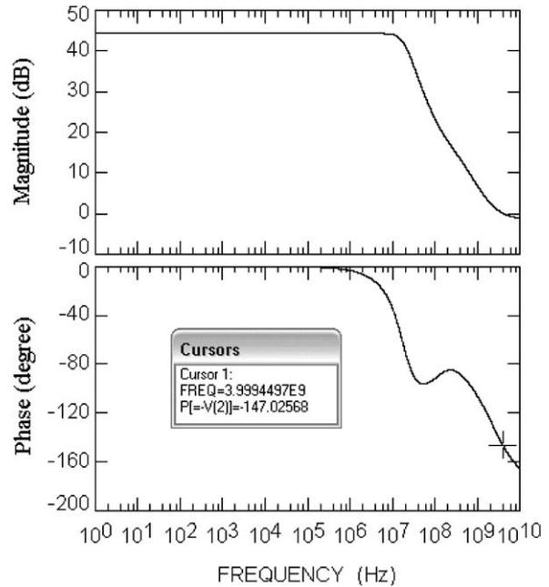
Fig. 6. Open Loop frequency response of the circuit shown in Fig. 2.
