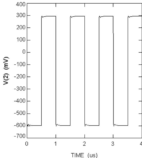
Fig. 13. The transient response of the circuit shown in Fig. 8.
