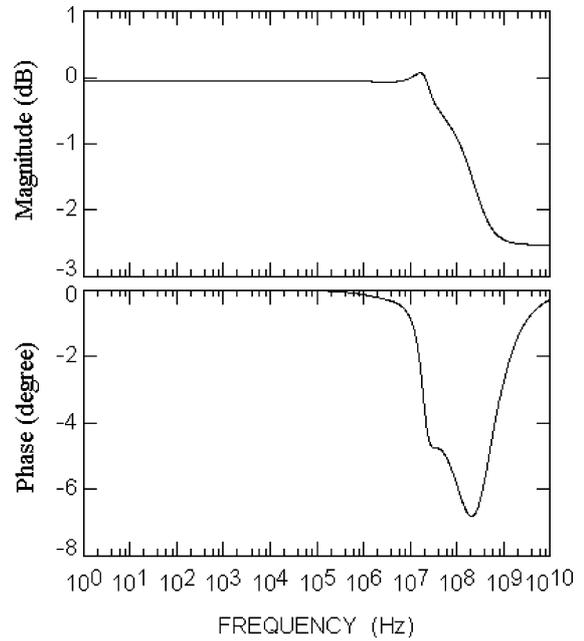
Fig. 10. Frequency characteristics of the open circuit voltage transfer gain between  $Y$  and  $X$  ( $V_X/V_Y$ ) for the circuit shown in Fig. 8.
