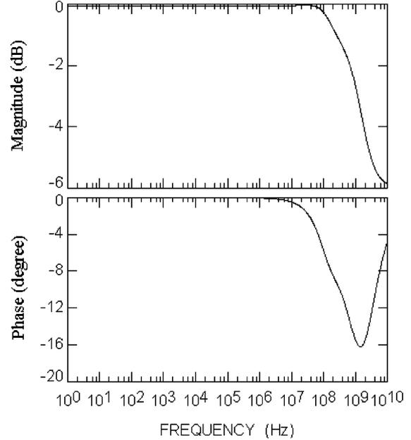
Fig. 4. Frequency characteristics of the open circuit voltage transfer gain between Y and X ( $V_X/V_Y$ ) for the circuit shown in Fig. 2.
