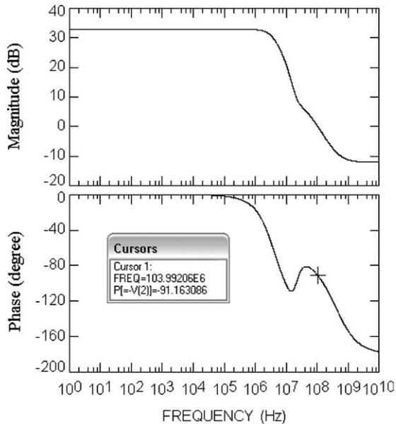
Fig. 12. Open Loop frequency response of the circuit shown in Fig. 8.
