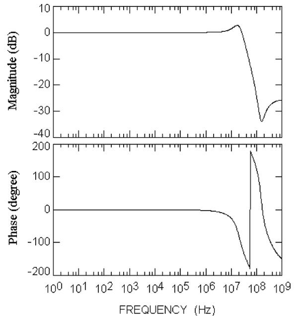
Fig. 11. Frequency characteristics of the short circuit current transfer gain between  $X$  and  $Z^+$  ( $I_Z^+/I_X$ ) for the circuit shown in Fig. 8.
