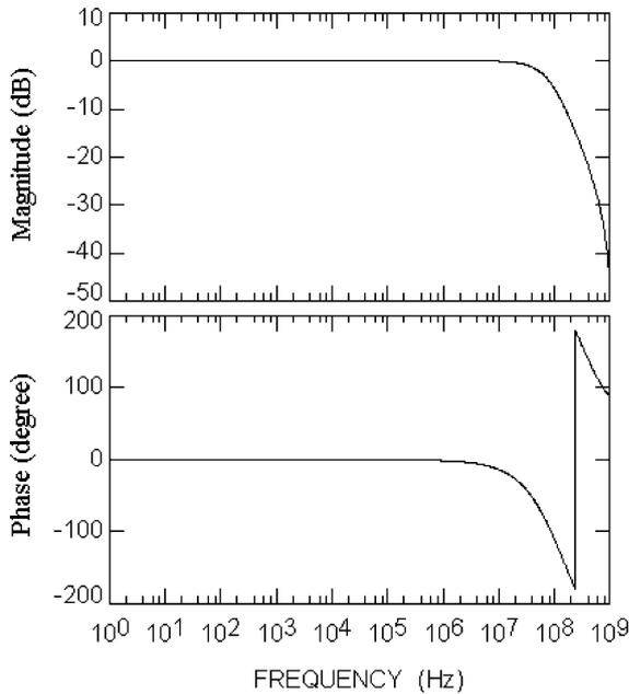
Fig. 5. Frequency characteristics of the short circuit current transfer gain between  $X$  and  $Z^+$  ( $I_Z^+/I_X$ ) for the circuit shown in Fig. 2.
