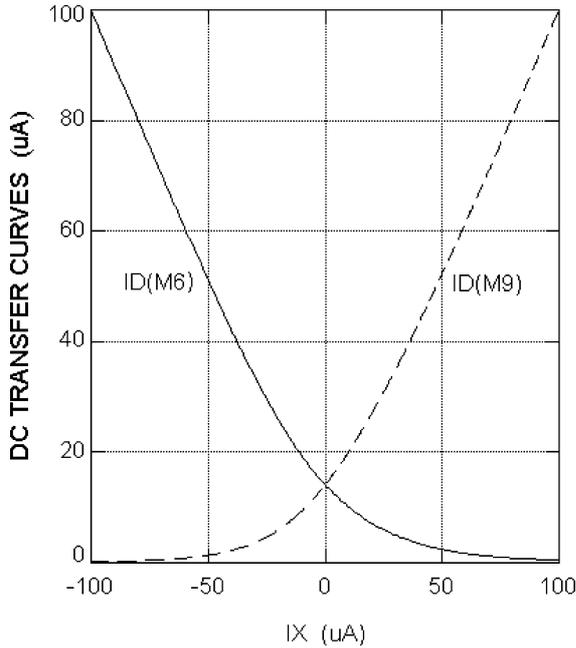
Fig. 9. The currents through  $M_6$  and  $M_9$  (push-pull).
