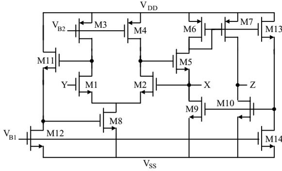
Fig. 8. Low power version of the new wide band CCII.
