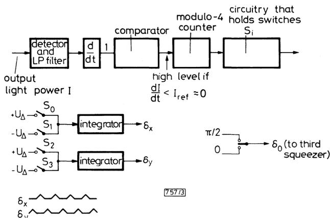
**Fig. 3** Implementation of electronic system for deriving the control signals  $\delta_x$ ,  $\delta_y$  and  $\delta_0$  from the polarised output light power  $\pm U_\Delta$  are direct voltages
