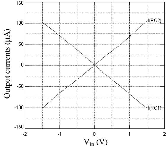
Fig. 7. Output currents of the extended linearity floating transconductor stage.
