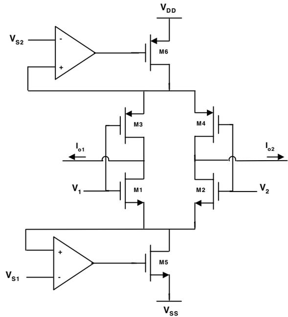
Fig. 2. The proposed transconductor circuit with feedback amplifiers.
