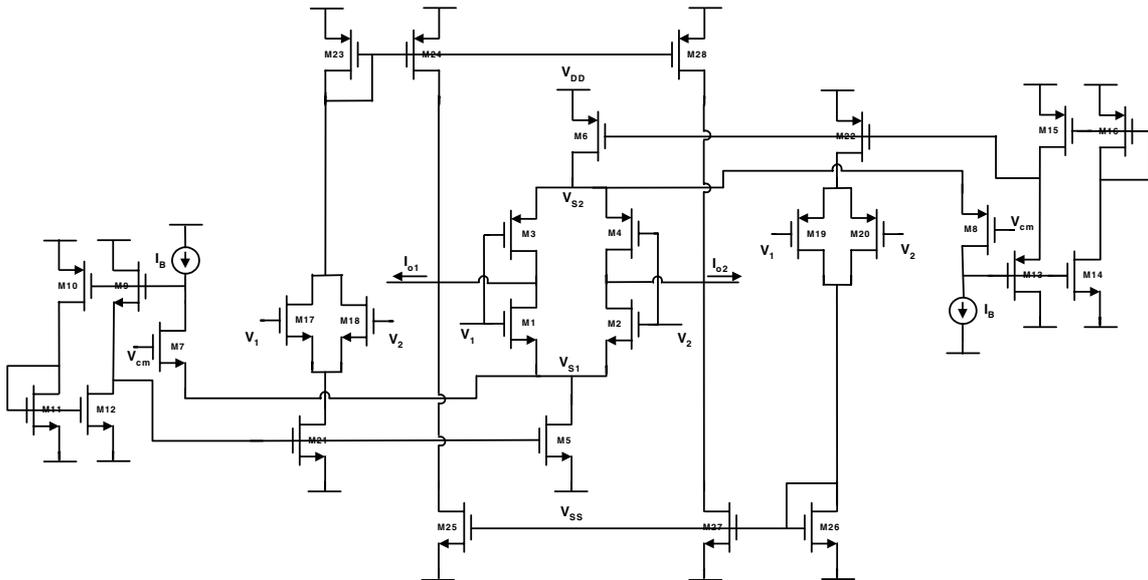
Fig. 5. Overall circuit diagram of the proposed low distortion transconductor.
