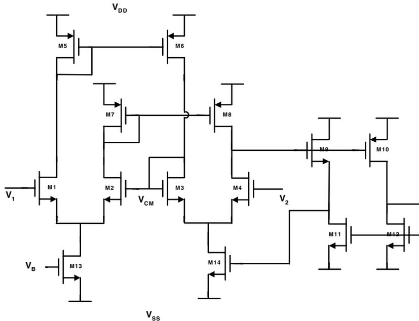
Fig. 4. Common mode estimator circuit [7].
