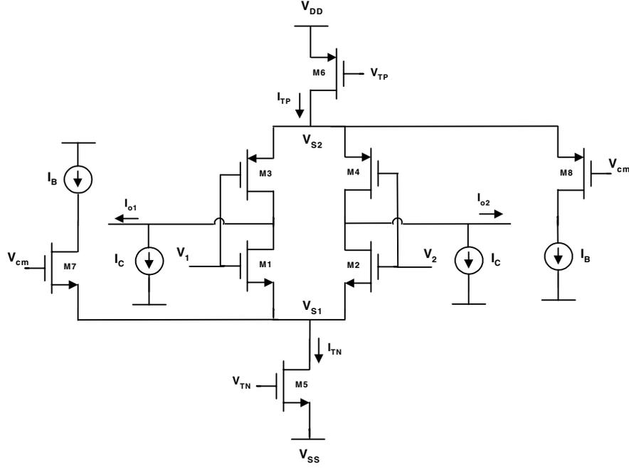
Fig. 3. The proposed transconductor circuit with the current feedback action.
