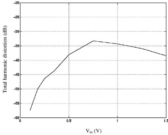
Fig. 10. THD plot versus the input amplitude.
