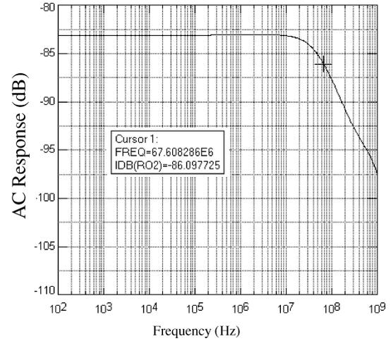
Fig. 12. Frequency response of the proposed transconductor.
