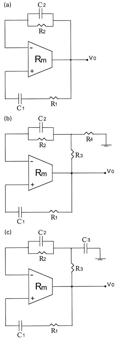
Fig. 3. Three single OTRA oscillator circuits.
