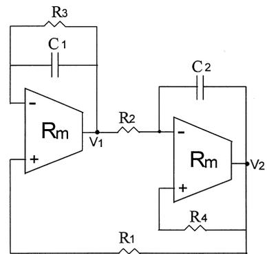
Fig. 4. Two OTRA oscillator circuit with independent control on the frequency of oscillation.
