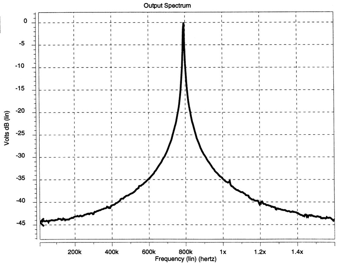
Fig. 9. (a) The output waveform of the oscillator of Fig. 3(c). (b) The frequency spectrum of the oscillator of Fig. 3(c).
