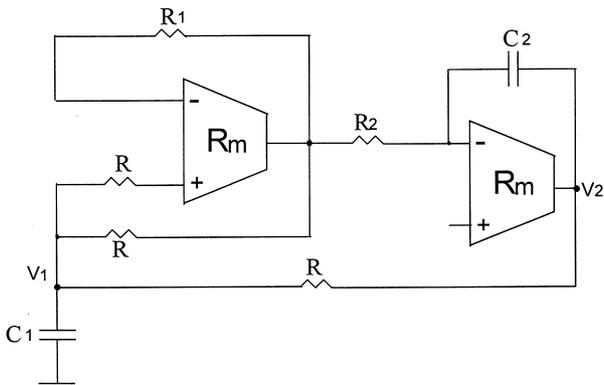
Fig. 6. An oscillator based on a novel grounded inductor using two OTRAs.
