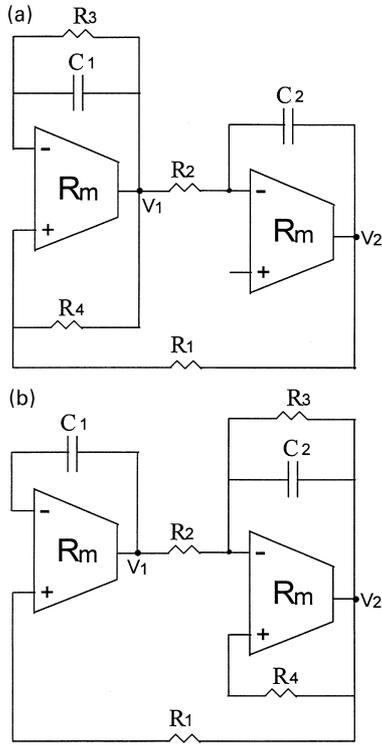
Fig. 5. Two equivalent quadrature oscillators.
