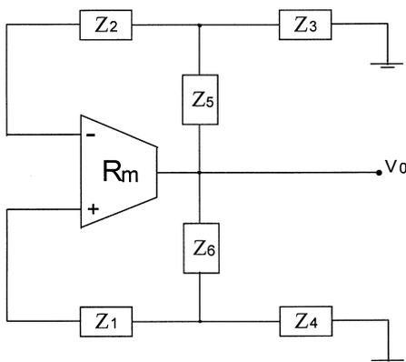
Fig. 2. The single OTRA generalized oscillator.
