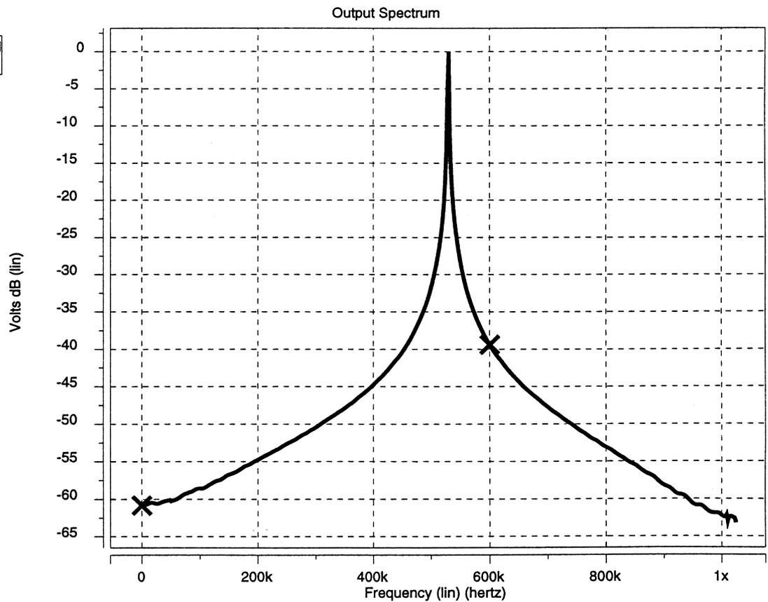
Fig. 7. (a) The output waveform of the oscillator of Fig. 3(a). (b) The frequency spectrum of the oscillator of Fig. 3(a).
