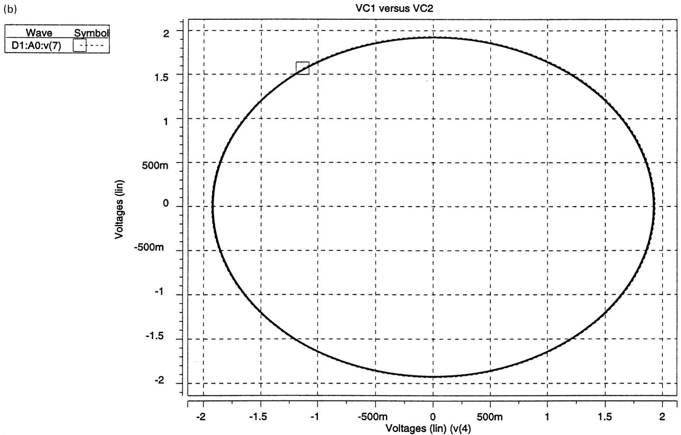
Fig. 10. (a) The output waveform of the oscillator of Fig. 5(b). (b) The voltage  $V_1$  versus  $V_2$  of the oscillator of Fig. 5(b).
