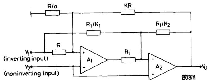
Fig. 1 Proposed differential VCVS
