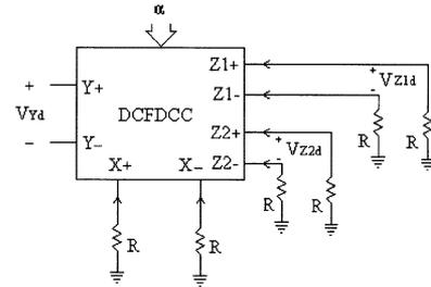
Fig. 18. DCFDCC-based VGA.
