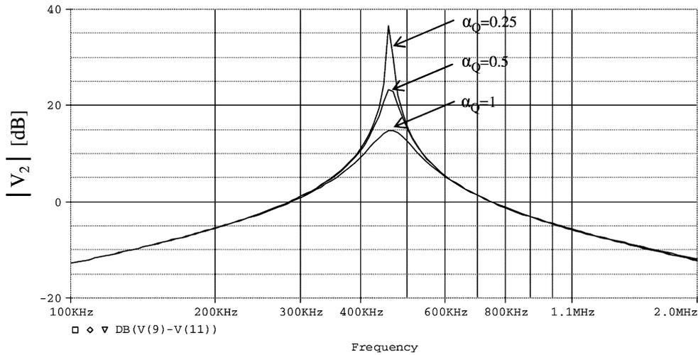
Fig. 15. Magnitude response the differential voltage bandpass output (different  $Q$  and the same  $f_0$  :  $f_0 = 450$  kHz).
