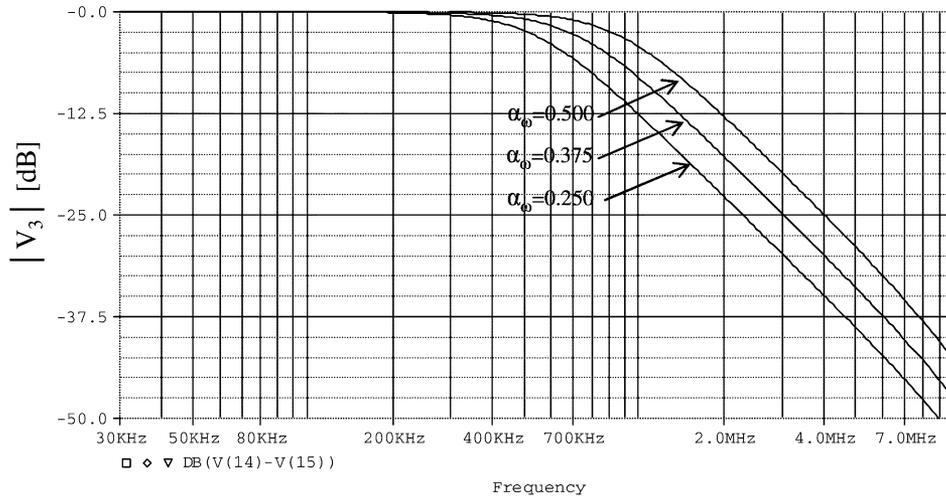
Fig. 12. Magnitude response the differential voltage low-pass output.
