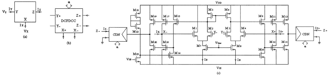
Fig. 3. (a) Symbol of the single-ended CCII. (b) Symbol of the first realization of the DCFDCC. (c) CMOS circuit of the first realization of the DCFDCC.
