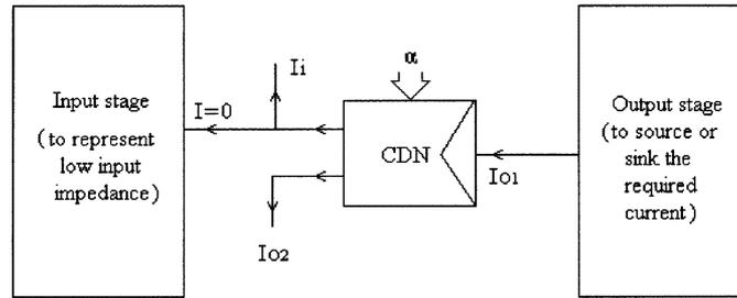
Fig. 7. Basic idea of the current gain approach.
