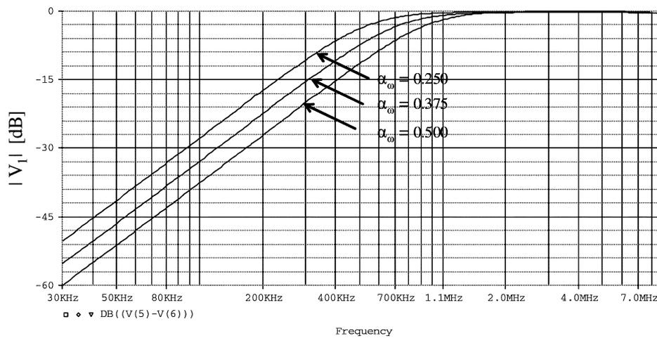
Fig. 13. Magnitude response the differential voltage high-pass output.
