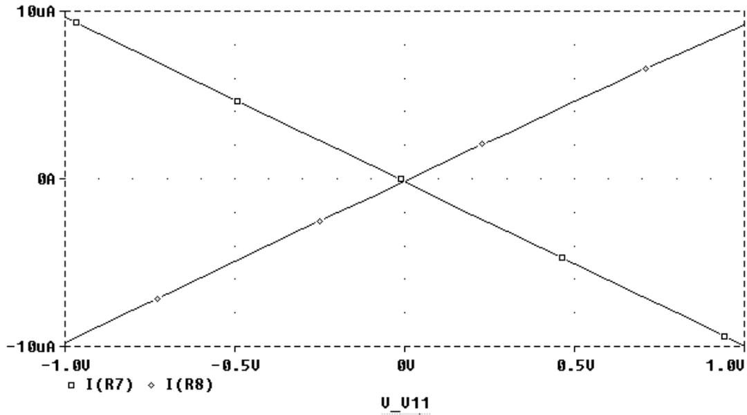
Fig. 9. The currents  $I_Y$  versus  $I_X$  of the CCIII+.
