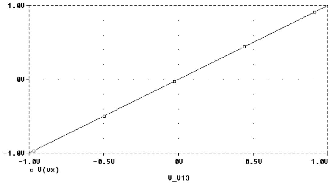
Fig. 7. The DC characteristics at node X for the proposed CCII+.
