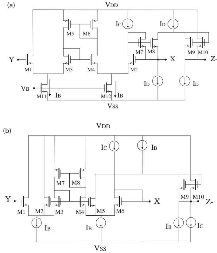
Fig. 4. (a) The circuit configuration of the proposed CCII-. (b) Another proposed circuit configuration of the CCII-.
