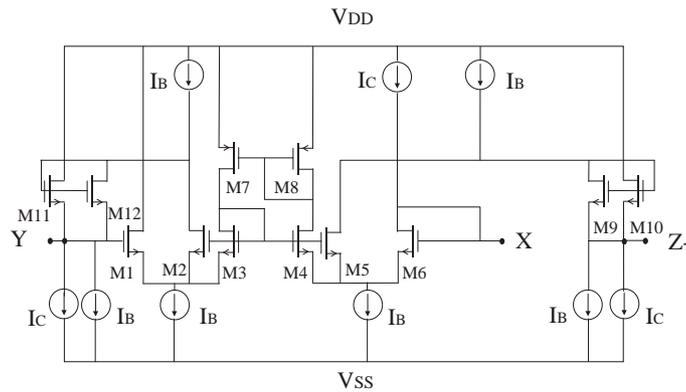
Fig. 6. The circuit configuration of the proposed CCIII-.
