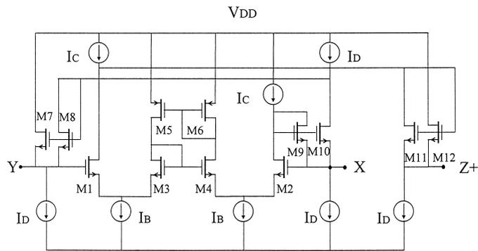
Fig. 5. The circuit configuration of the proposed CCIII+.
