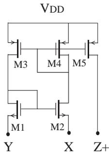
Fig. 1. The circuit configuration of the CCI+.
