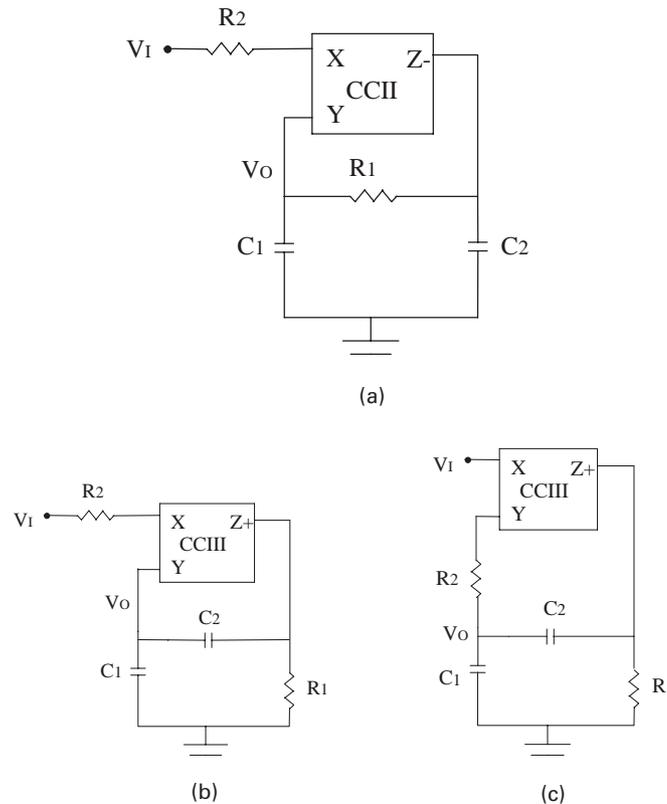
Fig. 10. (a) The low pass filter configuration using CCII-. (b) and (c) Two equivalent low pass filter configurations using CCIII+.
