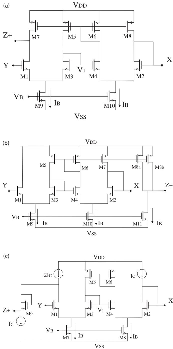
Fig. 3. (a) The circuit configuration of the proposed CCII+. (b) The circuit configuration of the modified CCII+. (c) The improved circuit configuration of the proposed CCII+ for better current following action.
