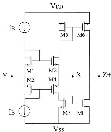
Fig. 2. The basic CCII based on the use of two complementary CCI circuits [2].
