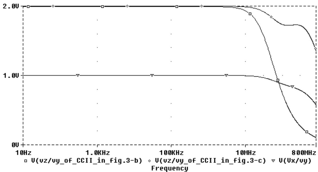
Fig. 8. The frequency characteristics of the voltage transfer functions using CCII+.
