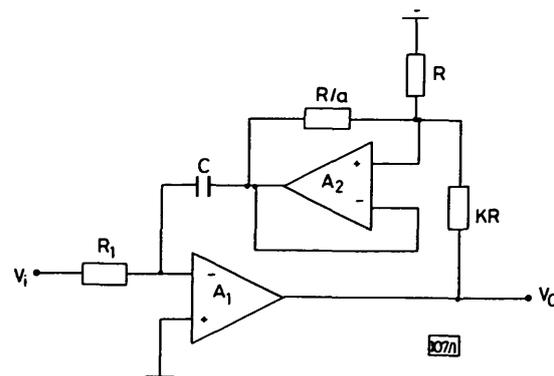
**Fig. 1** Proposed phase lead inverting integrator
