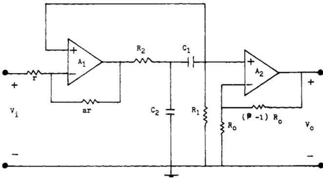
Fig. 1. A new canonic RC bandpass filter.
