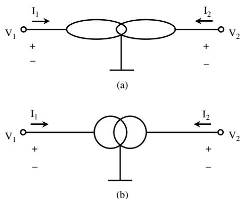
Fig. 2. The symbolic representations of (a) the voltage mirror (b) the current mirror.
