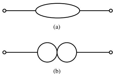
Fig. 1. The symbolic representations of (a) the nullator (b) the norator.
