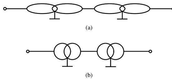
Fig. 3. (a) Nullator representation using the voltage mirror. (b) Norator representation using the current mirror.
