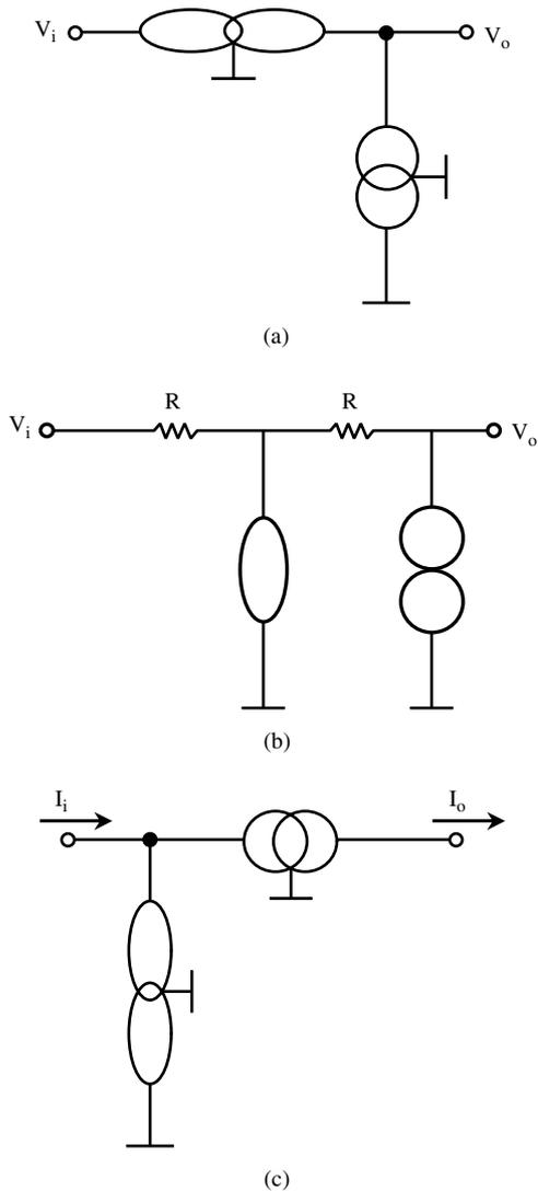
Fig. 6. (a) The voltage inverter mirror representation. (b) Nullor-based voltage inverter representation. (c) The current inverter mirror representation.
