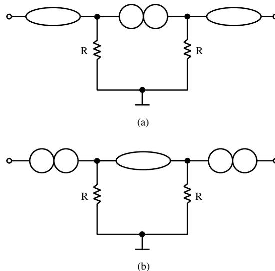
Fig. 4. Nullor based (a) voltage mirror representation (b) current mirror representation.
