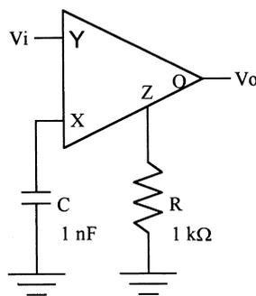
Fig. 2. The non-inverting differentiator used in testing the different macro-models.
