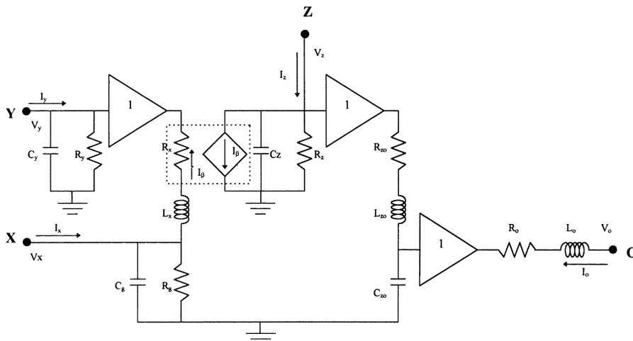
Fig. 10. The second proposed CFOA macromodel.
