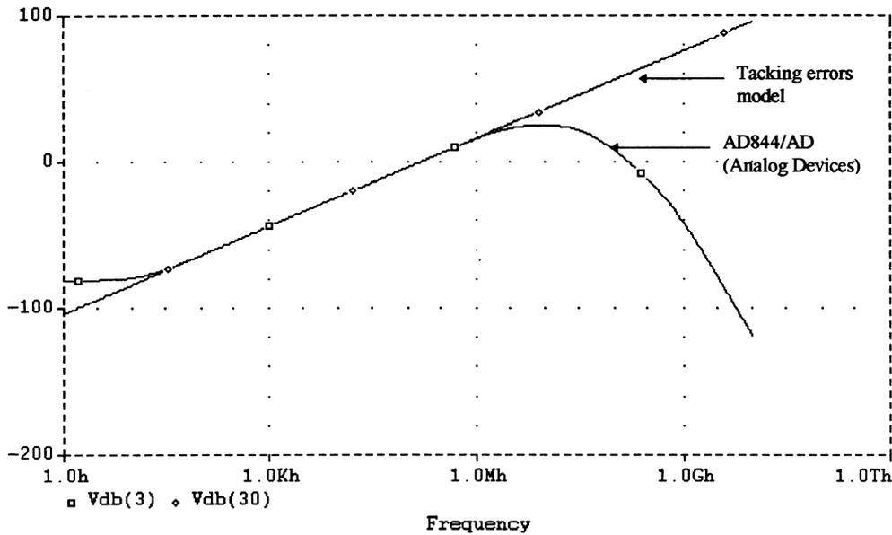
Fig. 3. The simulated response of the non-inverting differentiator shown in Fig. 2 for both the tracking errors model and the AD844/AD.
