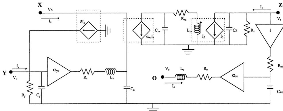
Fig. 6. The CFOA macromodel proposed in Ref. [8].
