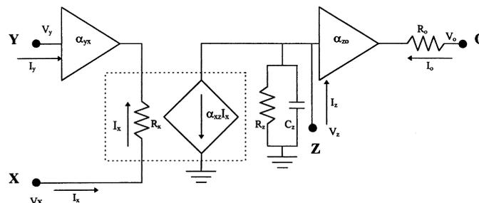
Fig. 4. A simple modeling of the non-idealities of the CFOA including the dominant parasitic effect.
