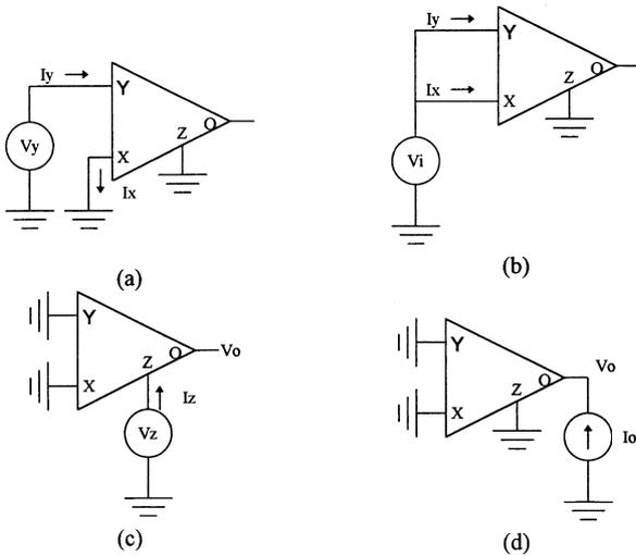
Fig. 11. The circuit configurations used in measuring the parameters of the second proposed macromodel: (a) Measuring  $R_y$ ,  $C_y$ ,  $R_x$  and  $L_x$ ; (b) measuring  $R_g$  and  $C_x$ ; (c) measuring  $R_z$ ,  $C_z$ ,  $R_{z0}$ ,  $L_{z0}$  and  $C_{z0}$ ; and (d) measuring  $R_o$  and  $L_o$ .
