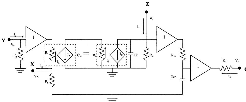
Fig. 8. The first proposed CFOA macromodel.
