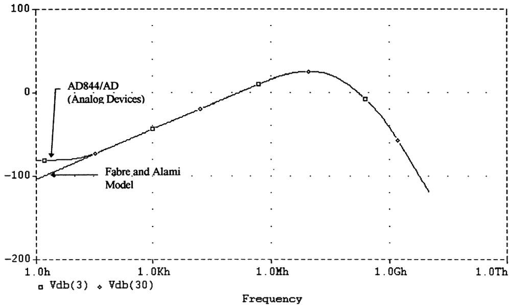
Fig. 7. The simulated response of the non-inverting differentiator shown in Fig. 2 for both the model presented in [1] and the AD844/AD.
