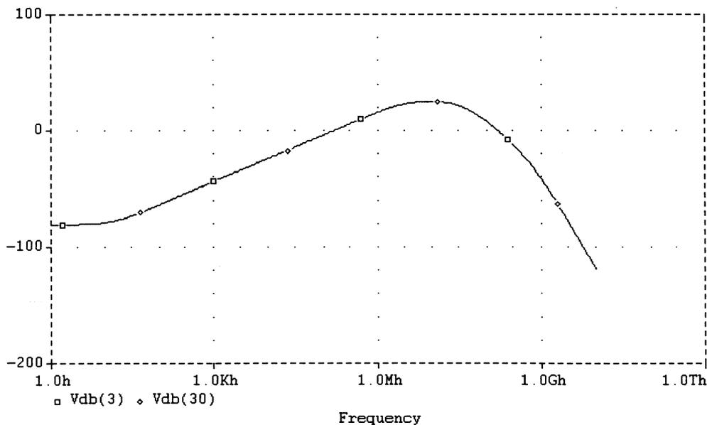
Fig. 12. The simulated response of the non-inverting differentiator shown in Fig. 2 for both the second proposed model and the AD844/AD.
