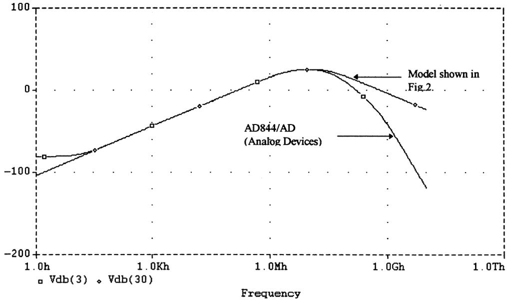
Fig. 5. The simulated response of the non-inverting differentiator shown in Fig. 2 for both the model shown in Fig. 4 and the AD844/AD.
