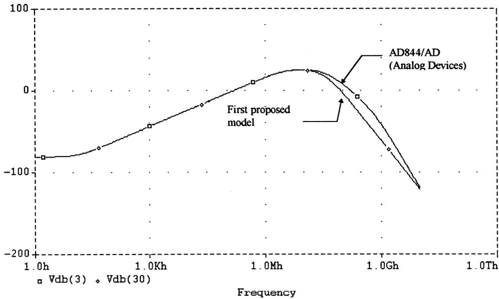
Fig. 9. The simulated response of the non-inverting differentiator shown in Fig. 2 for both the first proposed model and the AD844/AD.
