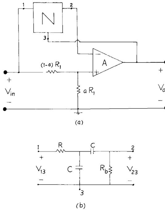
Figure 1. A single OA nonminimum phase network, (a) general configuration, (b) network N
