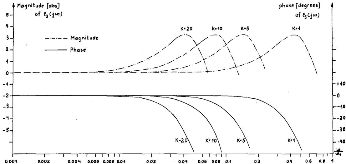
Fig. 3 Calculated magnitude and phase characteristics of  $\epsilon_3(j\omega)$  plotted versus  $\omega/\omega_1$ , with  $K$  taken as a parameter.
