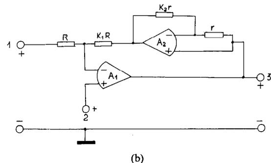
Fig. 1 (a) The uncompensated three-port opamp VCVS active building block. (b) The proposed compensated three-port opamp VCVS.
