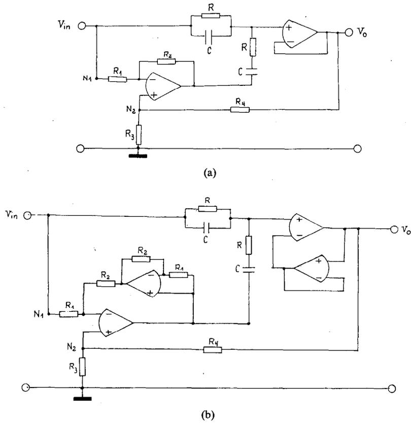
Fig. 5 (a) Wilson's all-pass filter section. (b) The modified all-pass filter section.
