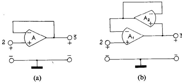
Fig. 2 (a) The uncompensated voltage follower. (b) The compensated voltage follower.
