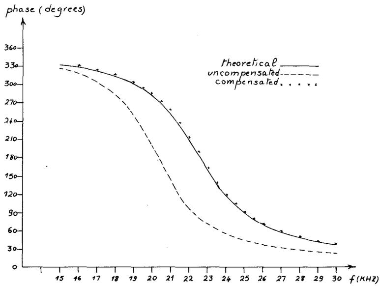
Fig. 6 Phase frequency response of the all-pass filters of Fig. 5(a) and (b).
