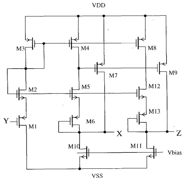
Fig. 4. The voltage conveyor circuit.
