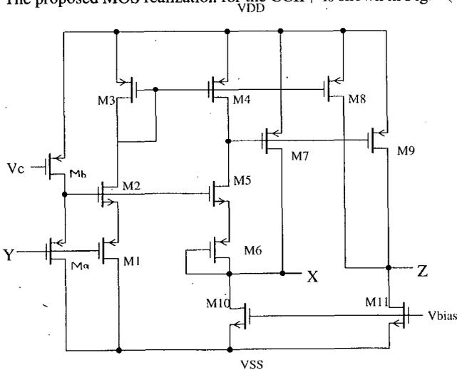
Fig. 2. The compensated current conveyor circuit.
