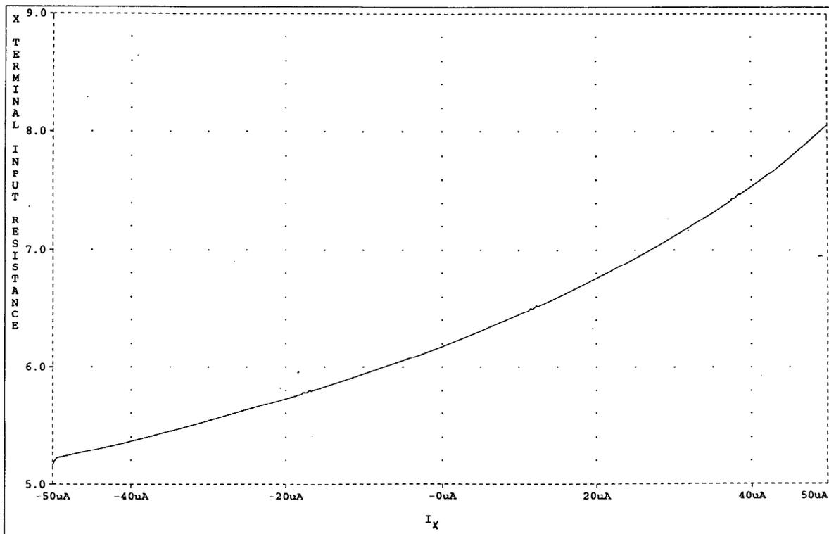
Fig. 6. The X terminal input resistance versus  $I_X$ .
