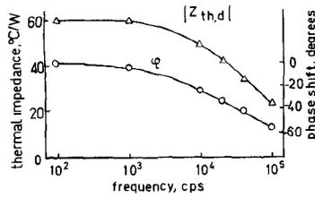
Fig. 3. Temperature difference of the b-e junctions of  $Q_3$  and  $Q_4$  per watt of power change in the collector dissipation of  $Q_3$  versus frequency.
