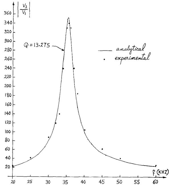
Fig. 2. Bandpass characteristics.
