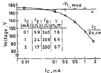
Fig. 4. The modified intercept voltage  $V_{I,mod}$  of a CA3046 transistor versus the collector current. For comparison, the quotient  $I_C/g_{0,cm}$  of the current mirror is also represented.
